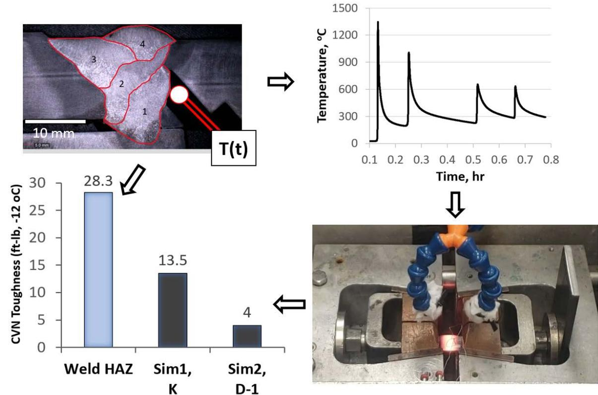
*Figure 1: Closed loop validation compares welding to physical simulation directly*
