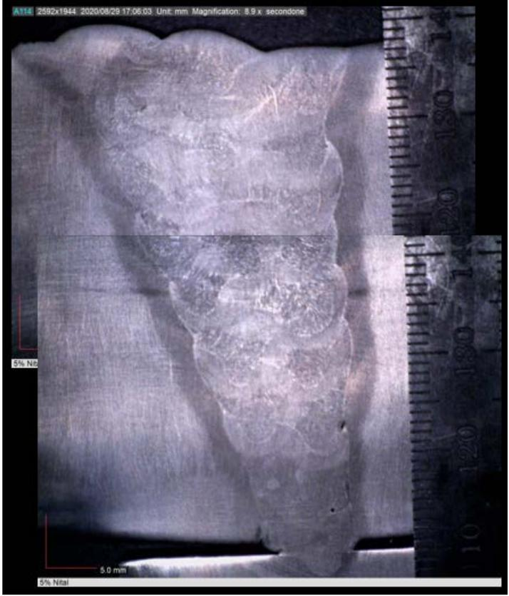
Figure 1: Weld Cross Section
