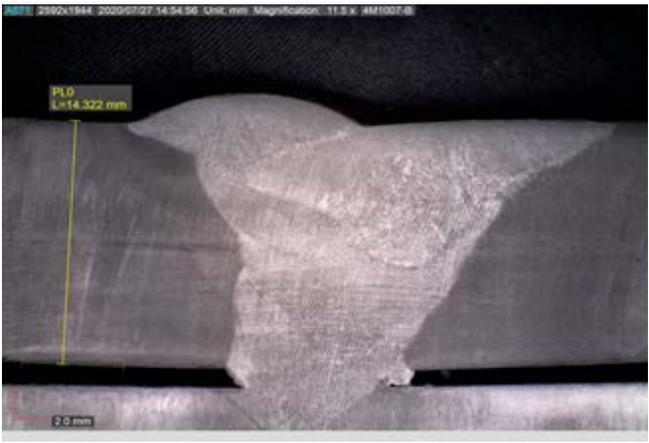
Figure 2: Weld Cross Section
