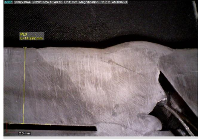
Figure 3: Weld Cross Section w/ TC
