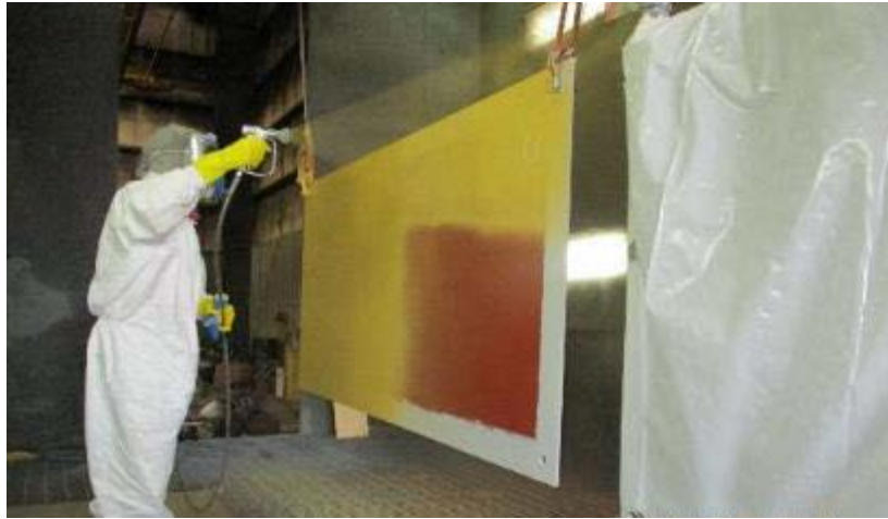
Intergard 267 and Sigmacover 520 Systems Completed at BAE JSR in December 2019 Panels Submerged in January 2020
