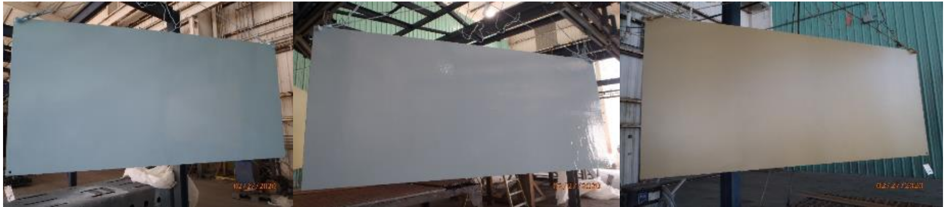
Fast Clad Primer and Hempel 47183 Systems Completed in March 2020
