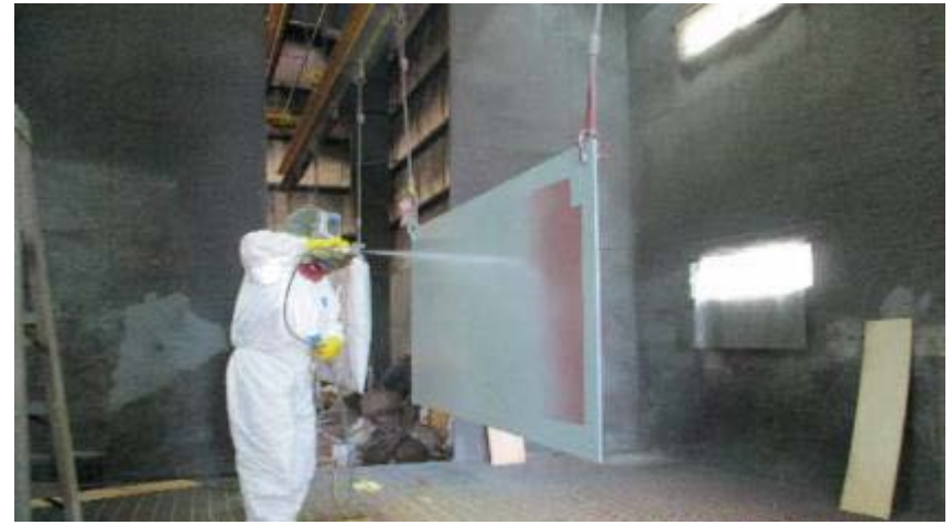
Intergard 267 and Sigmacover 520 Systems Completed at BAE JSR in December 2019 Panels Submerged in January 2020
