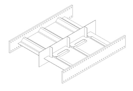
Swaged Bulkhead Above Angle-stiffened Bulkhead, Fully Connected, w/Outfitting Penetrations
