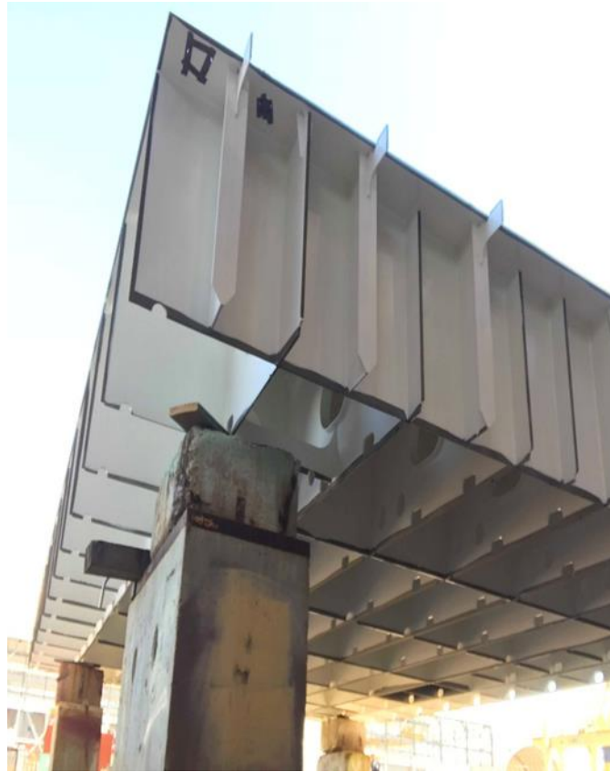
Figure 5. Unit After Coating with Type VI Primer in Blast and Paint Hall.
