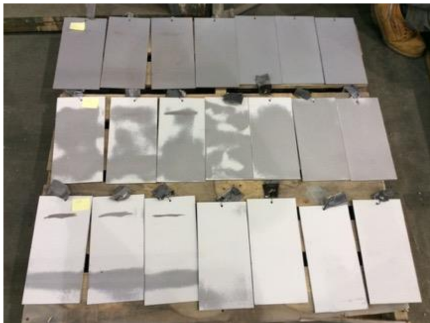
Figure 5. Panels after Surface Preparation
