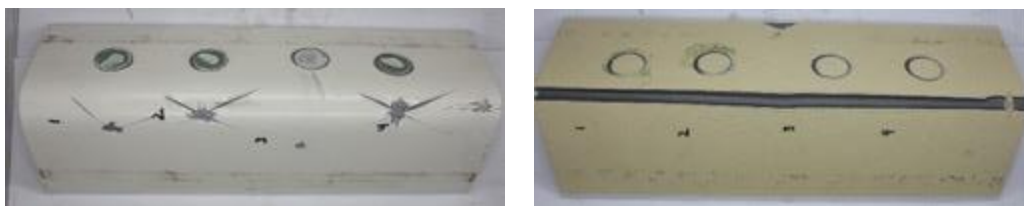
Figure 17. Panels 10YA1 (left) and 5A1 (right) after bend at 110 degrees
