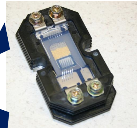
High power electronics assembly with large diameter wire bonds and high voltage encapsulant
