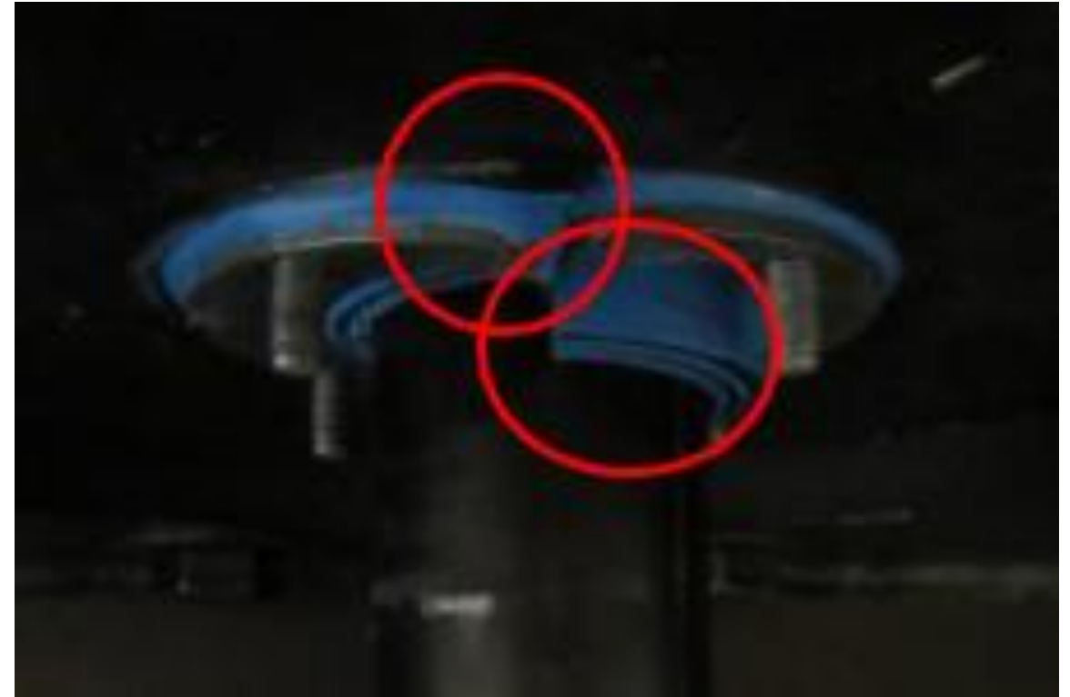
“Telescoping” of RS OMD, 10 lbs. added weight, hammer dropped from 5ft
