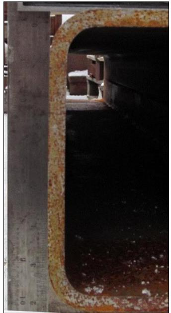
Figure 9. Symmetry in the HFRW Tube Deformation after Fatigue Testing
