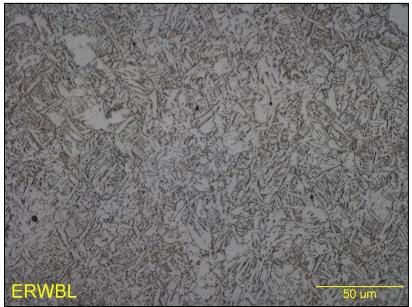
Figure 25. HFRW Weld at 500× Magnification
