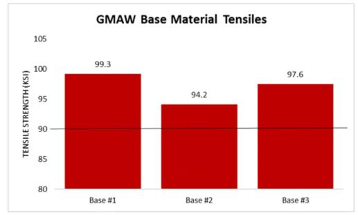
Figure 14. Tensile Test Graph for GMAW Base Material
