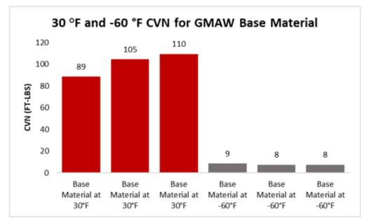
Figure 16. CVN Graph for GMAW Base Material Tested at 30°F and -60°F
