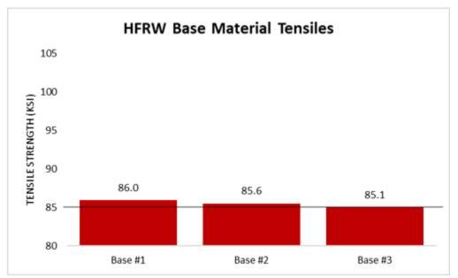
Figure 15. Tensile Test Graph for HFRW Base Material
