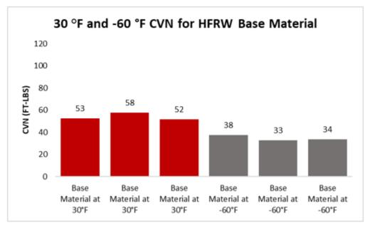
Figure 17. CVN Graph for HFRW Base Material Tested at 30°F and -60°F
