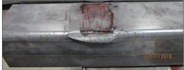
Figure 12. Cracking in HFRW Tube Showing Uniform Cracks in Two Corners
