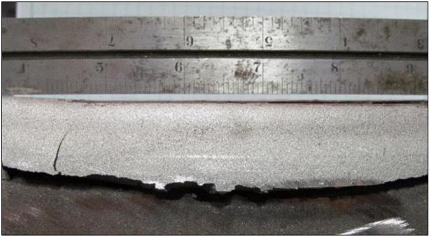
Figure 11. Up Close Side View of Cracking in GMAW Tube
