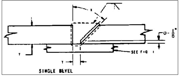
Figure 5. B1V.5 Weld Joint for GMAW Mechanical Test Weld Specimen
