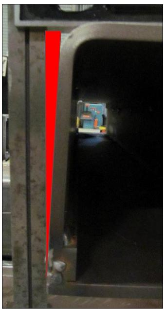
Figure 8. Residual Asymmetry in the GMAW Tube Deformation after Fatigue Testing
