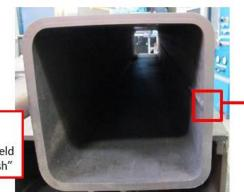
Impurities and molten metal squeezed out of weld joint is called "Flash"
