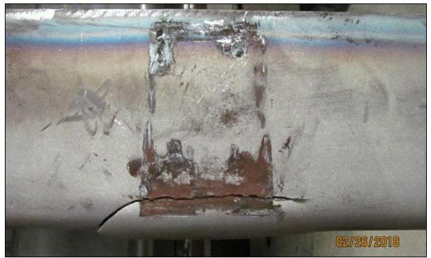
Figure 10. Large Failure Site Cracking in GMAW Tube
