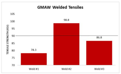
Figure 19. Tensile Test Graph for the GMAW Welds
