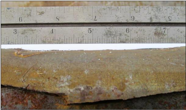
Figure 13. Up Close Side View of Cracking in HFRW Tube
