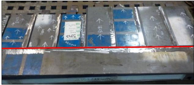
Figure 6. GMAW Mechanical Test Specimen Prepared for Welding
