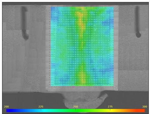
Figure 24. Vickers Hardness Map of the HFRW Tube Weld Joint
