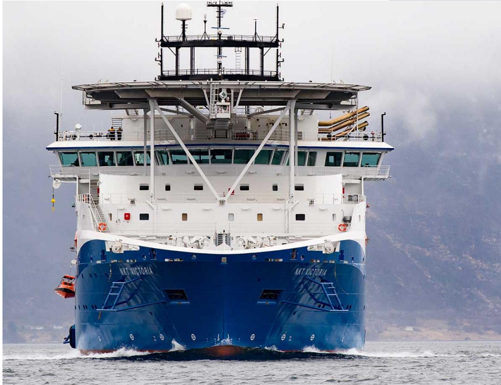
NKT VICTORIA – 9000t cable capacity
