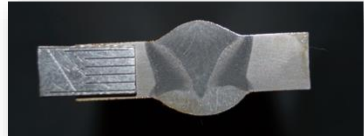
7 mm (SuperMIG – single pass)
