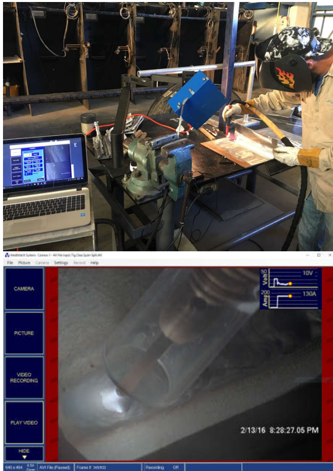
Figure 1: 3-D Goggles used during testing (Upper Left), Experimental setup prior to welding (Upper Right), View of welding when the system is in use (Lower Left), View of welding utilizing the camera system (Lower Right)
