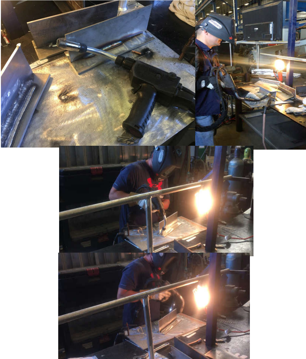
Figure 3: Aluminum welding gun and aluminum welds produced during testing (Upper Left), Blind welding of overhangs (Upper Left), Views of Blind welding of a 12-inch length before (Lower Left) and after (Lower Right) welding
