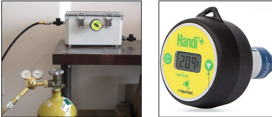
Figure 5. Inerted Container and Oxygen Monitor
