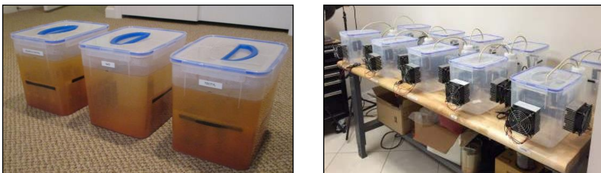
Figure 3. Immersion (left) and Atmospheric with and without Condensation (right) Testing
