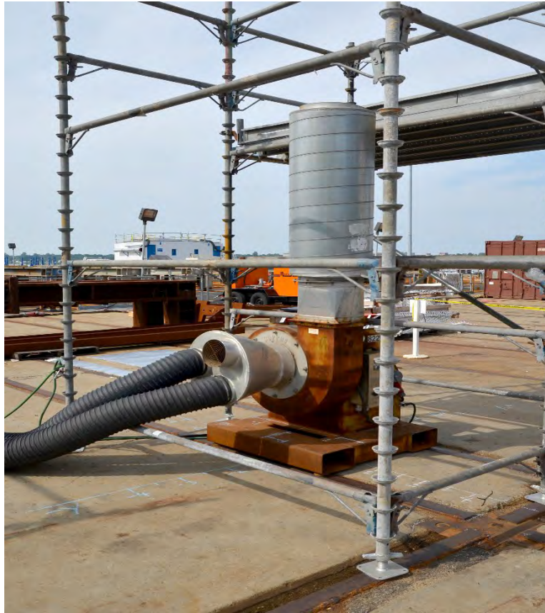
Figure 7 – Coppus TM-8 Blower (Shipyards ID 822)
