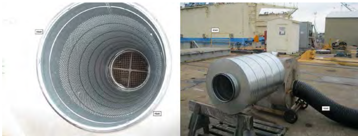
Figure 3 –Exhaust Silencer: Interior view (left photo) and the exterior view (right photo).
