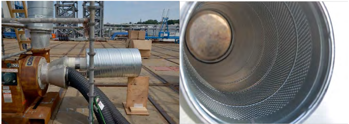
Figure 9 – Intake Silencer for Coppus TM-8: Exterior View (left photo) and Interior View (right photo)
