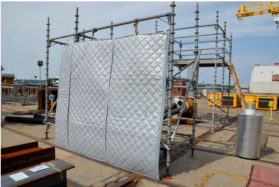
Figure 10- Acoustical curtain for Coppus TM-8, as tested
