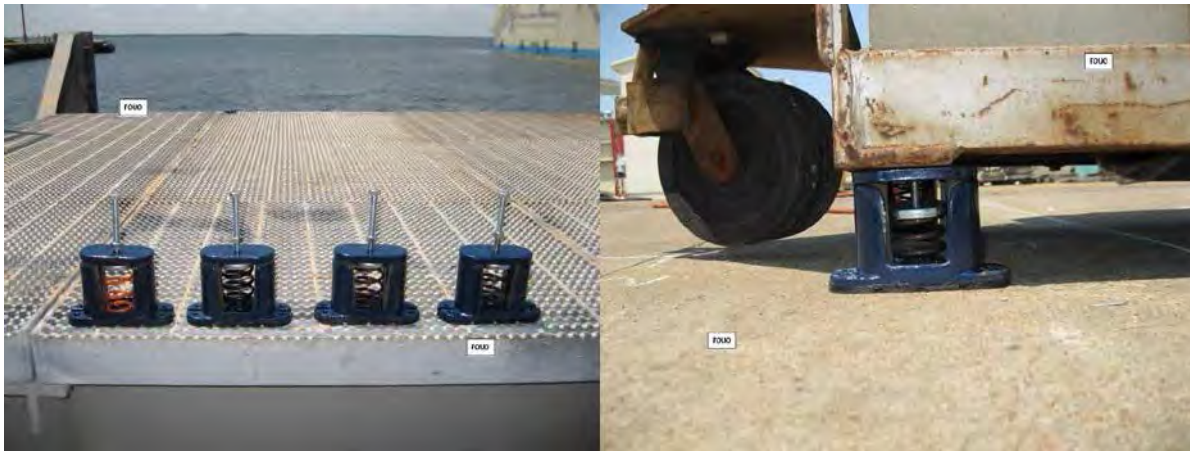
Figure 5 – Vibration Isolation mounts (left photo) are sized for the weight at each corner of the PVB and the photo on the right shows one mount with the full weight of the PVB on the spring mounts – wheels off the ground.
