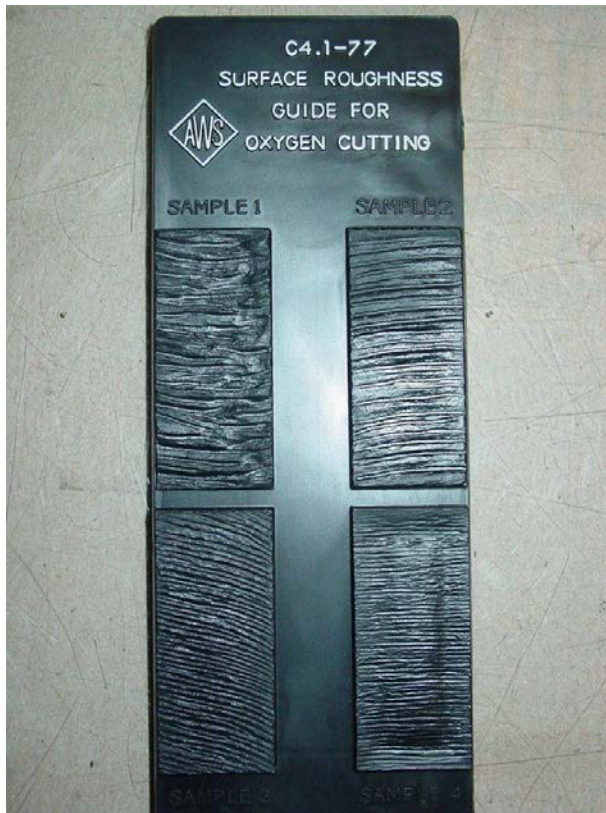
Figure 1 – Flame Roughness Guide for Oxygen Cutting
