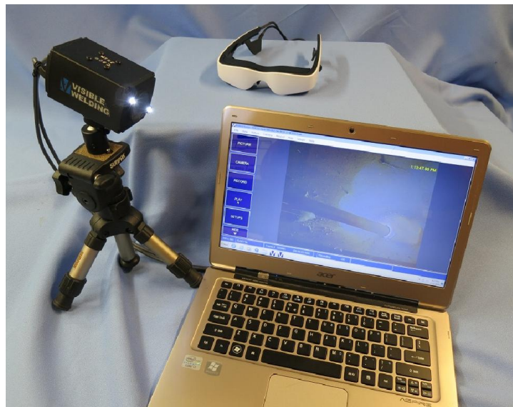
The test configuration combined a fully functional camera-head prototype with a PC performing all the functions of the belt-pack controller. The HD OLED video goggles are from Zeiss.
