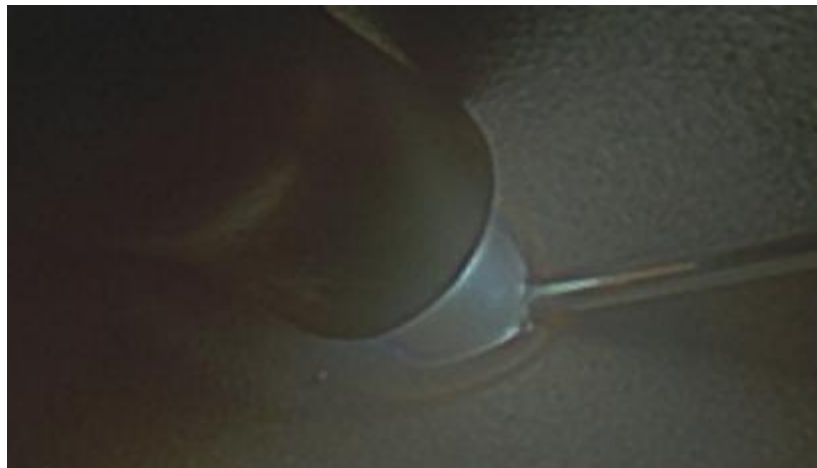
In-goggle view, as seen by the welder. With 10x optical zoom plus 8x digital zoom, the welder can choose their view.
