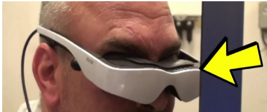
High-Def video goggles give the welder a close-up view of the weld.
