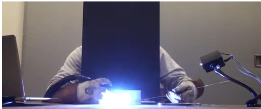
In the alpha field tests, a steel wall was used to block the view. The welder welds using the live video feed from the beta camera (on right in photo)
