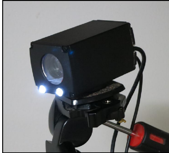
Beta camera on a tripod. The LEDs help illuminate the work during setup when arc is off.
