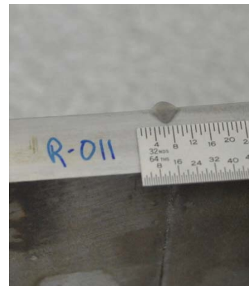
Figure 5. Top: fillet and butt welds made on DH-36 test material. Bottom left, fillet weld made at 59 ipm. Bottom right: macro of butt weld made at 59 ipm.
