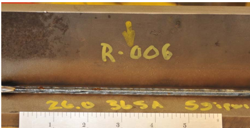
Figure 5. Top: fillet and butt welds made on DH-36 test material. Bottom left, fillet weld made at 59 ipm. Bottom right: macro of butt weld made at 59 ipm.
