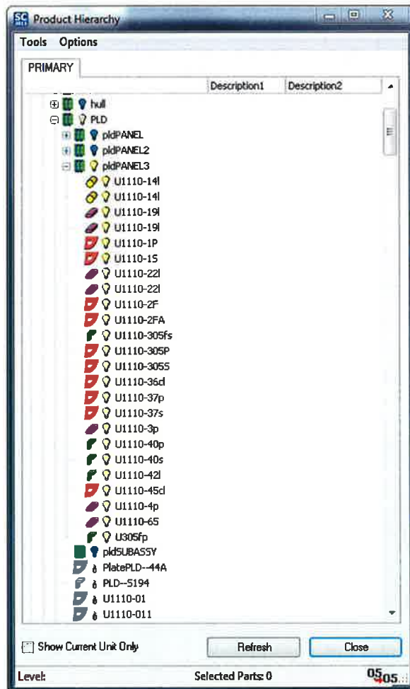
Figure 48: Example Sample Build Sequence from a ShipConstructor Product Hierarchy
