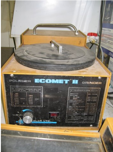
Figure 10. Diamond wheel polisher
