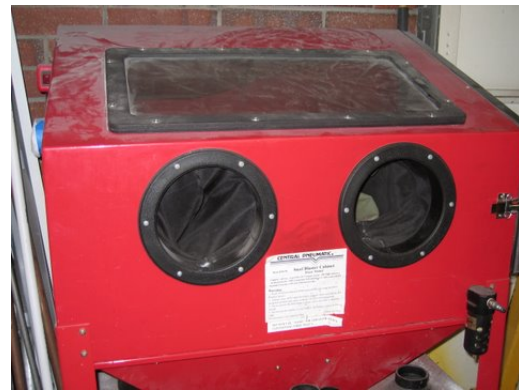
Figure 7. Sample grit blasting machine
