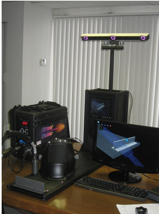
Figure 1. Full virtual welding system
