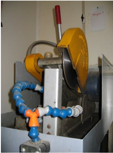
Figure 8. Abrasive cutoff wheel with auxiliary cooling system
