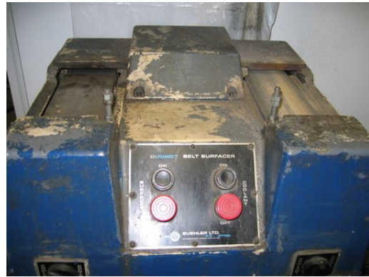
Figure 9. Large heavy grinding system for sample preparation
