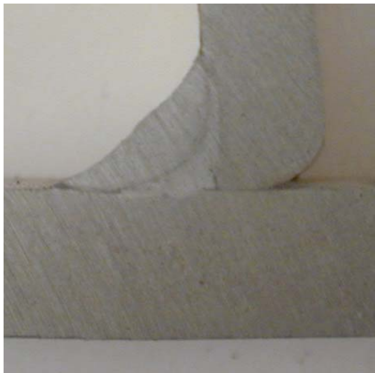
Figure 6.49: Cross-section Showing Penetration Profile of Benchmark Assembly4
