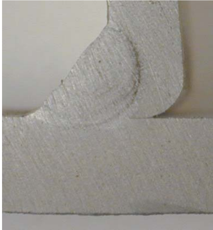
Figure 6.48: Cross-section Showing Penetration Profile of Benchmark Assembly3
