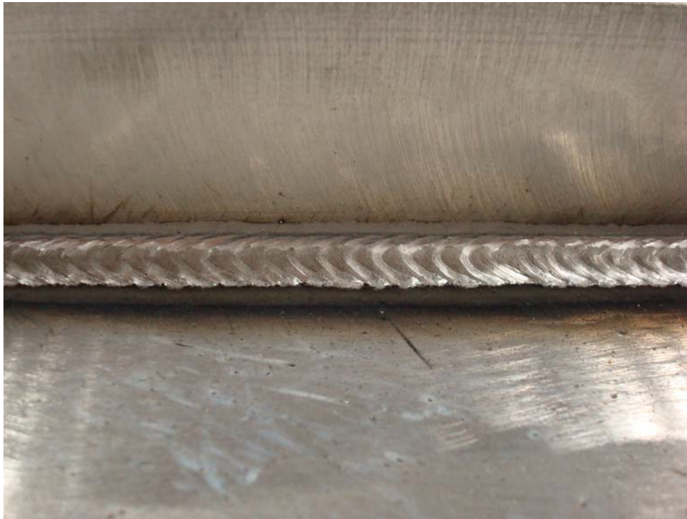
Figure 6.44: Weld Profile, Benchmark Assembly 4 (Pulse on Spray)
