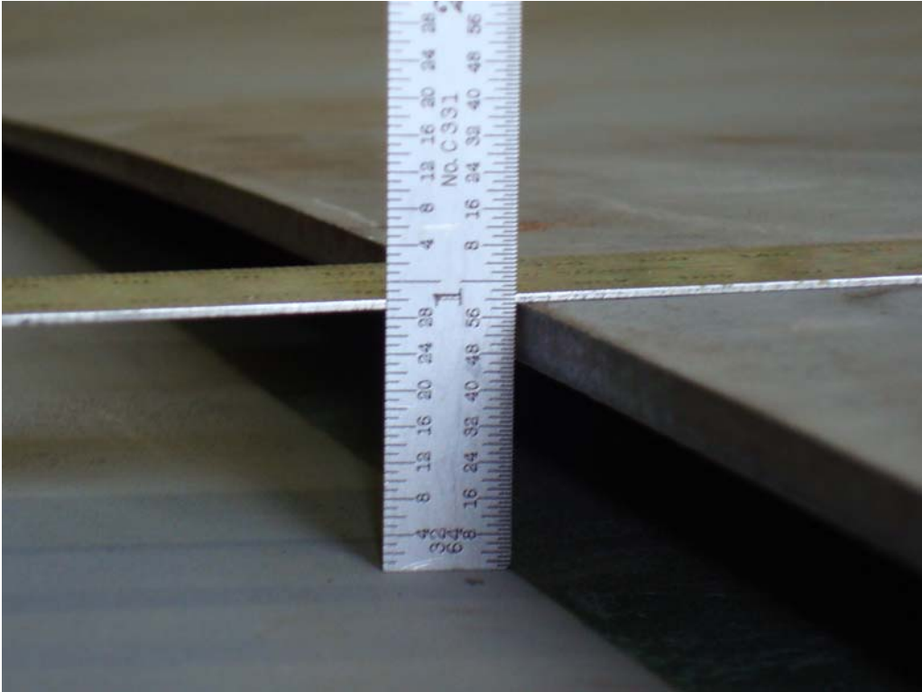
Figure 4.8: High Low in Plates before Pre-Tensioning
