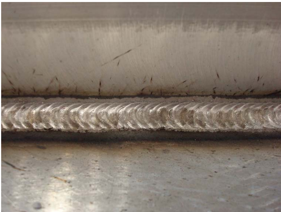
Figure 6.43: Weld Profile, Benchmark Assembly 3 (Pulse on Short)
