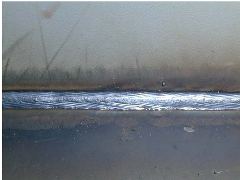
Figure 7.18: T-MCAW Weld Profile with 85Ar/15C02
