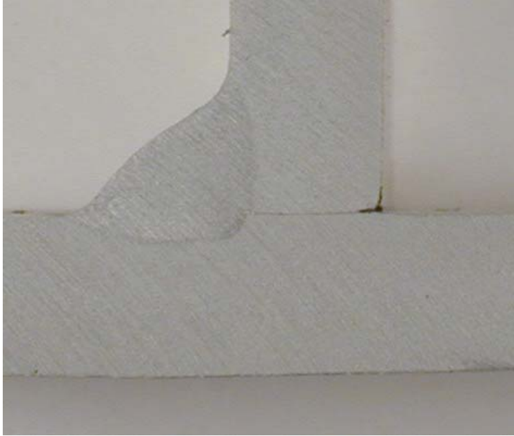
Figure 6.50: Cross-section Showing Penetration Profile of Assembly5
