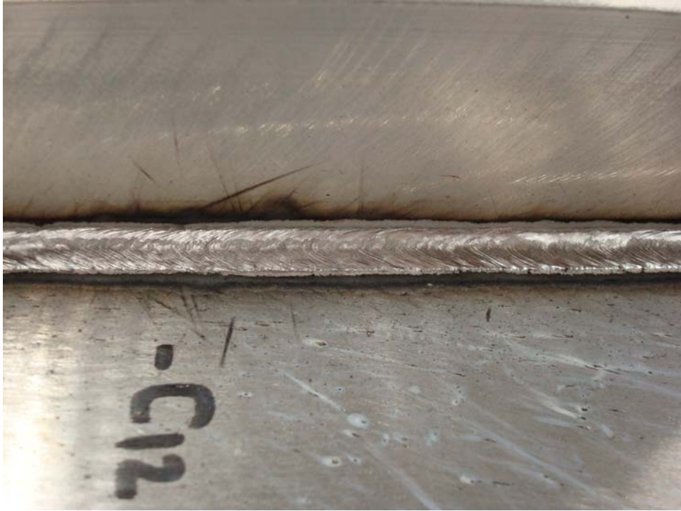
Figure 6.41: Weld Profile, Benchmark Assembly 1 (Conventional CV)
