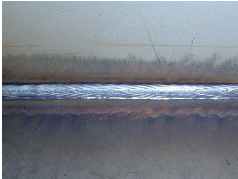
Figure 7.17: T-MCAW Weld Profile with 92Ar/8C02
