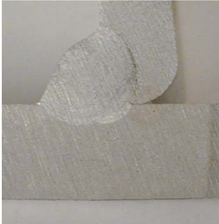
Figure 6.46: Cross-section Showing Penetration Profile of Benchmark Assembly1
