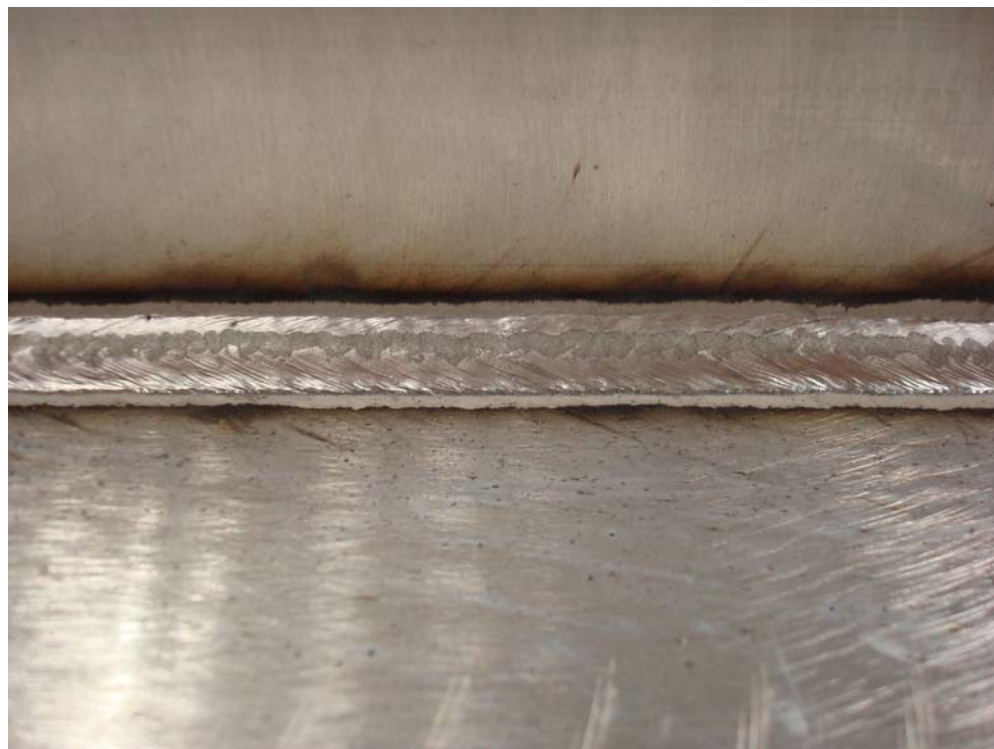
Figure 6.45: Weld Profile, Benchmark Assembly 5 (Pulse)
