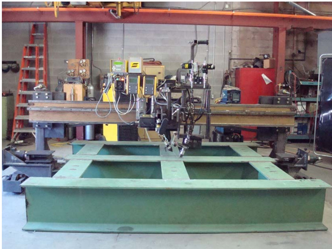
Figure 3.1: Welding Gantry and Frame Set-up
