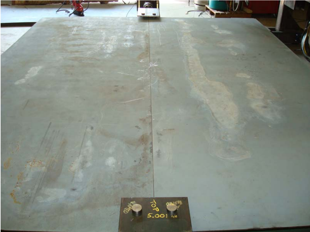
Figure 4.9: Fit-Up of Plates after Pre-Tensioning
