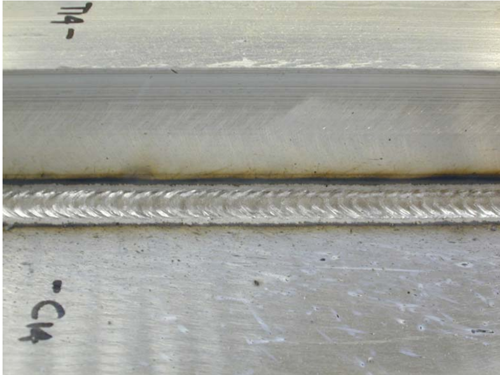
Figure 6.42: Weld Profile, Benchmark Assembly 2 (Pulse on Pulse)
