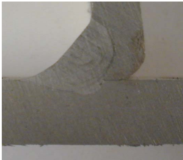
Figure 6.47: Cross-section Showing Penetration Profile of Benchmark Assembly2
