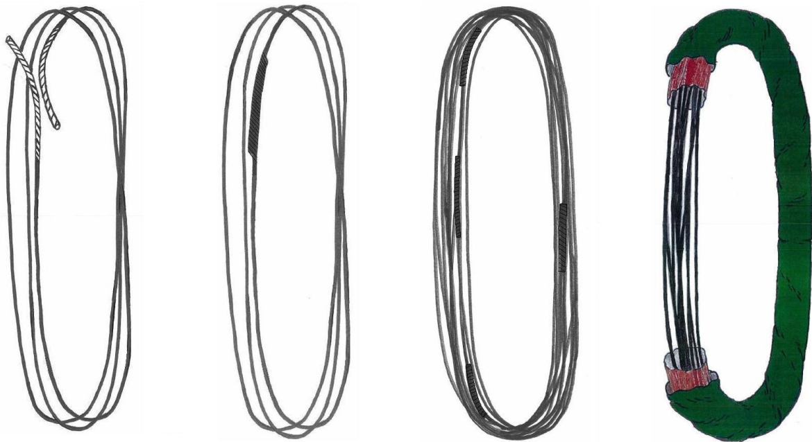
Figure 12: Component Construction of a Single Path Roundsliding
