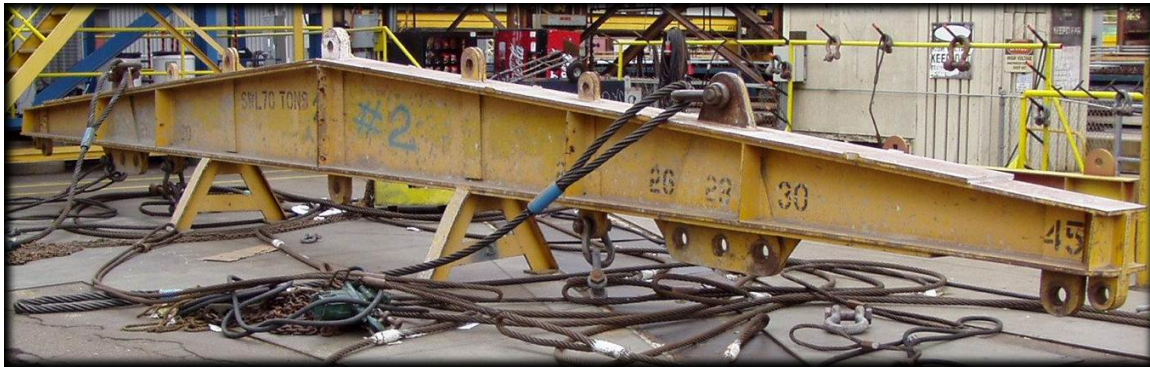
Figure 34: Single Web Girder Spreader Beam
