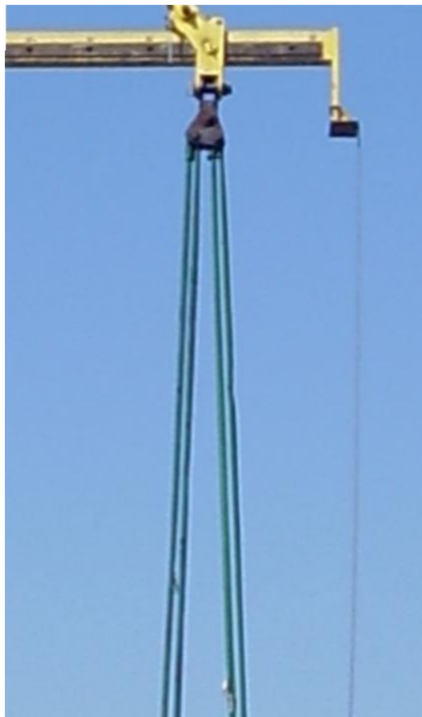
Figure 1. Load Sharing Device Near the End of Spreader Beam
