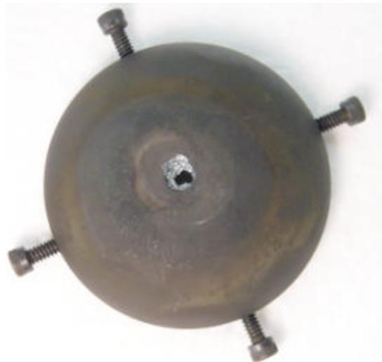
**Figure 18: Big Graphite Shield with eroded tip**
