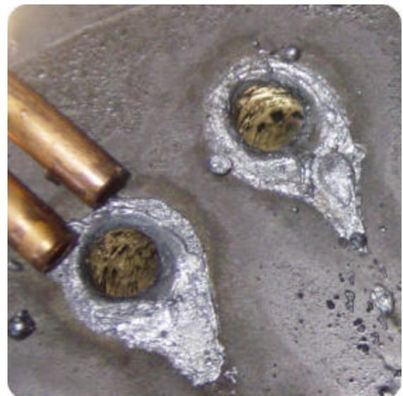
Figure 28: Quick Test #1 partial piercing (close-up)
