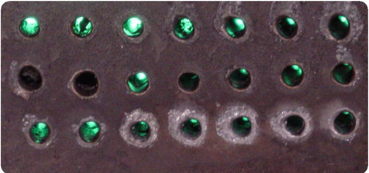
**Figure 34 Top view of the 21 continuous pierced holes made with the anti-spatter application using the side air jet piercing technique.**
