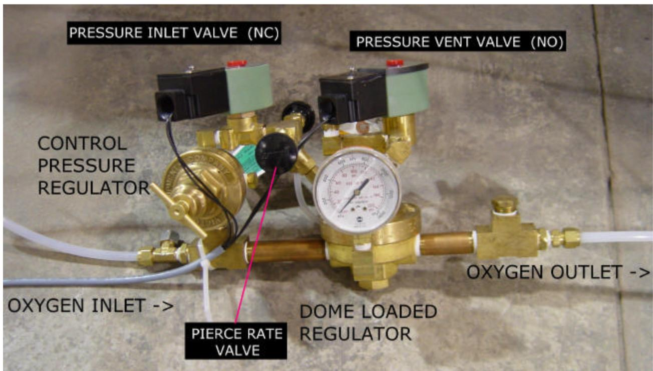
Figure 36: Labeled LASOX oxygen gas control assembly
