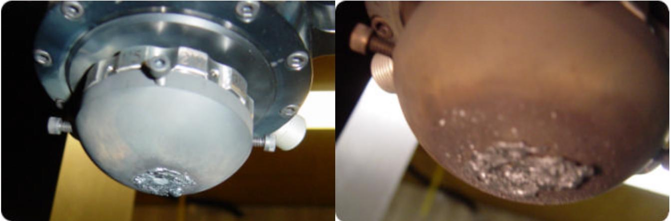
**Figure 16: Big Graphite Shield after piercing**
