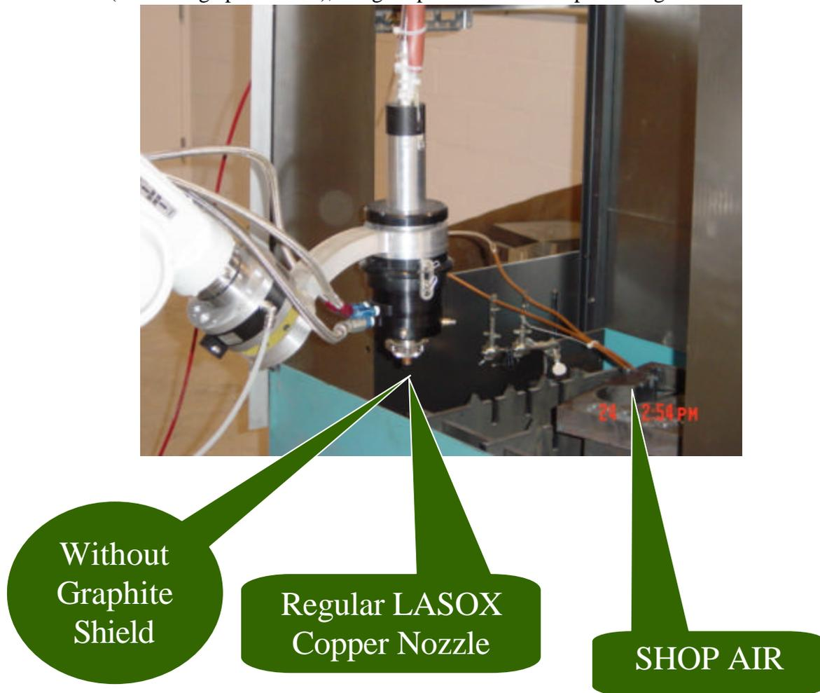
Figure 26: Quick Test #1 set-up
