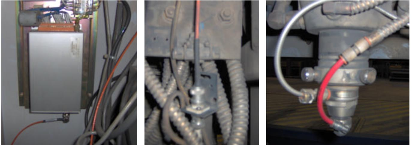
**Figure 39 - 41: Photo of the Precitec Height Sensing box, cable, and connection to head.**
