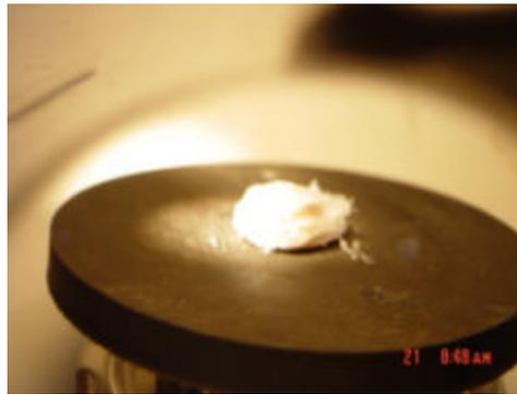
Figure 20: Gouping nozzle with anti-spatter grease.
