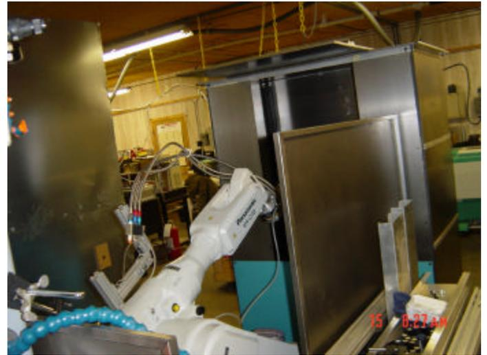
Figure 4: Robot w/LASOX Head and Protective Enclosure
