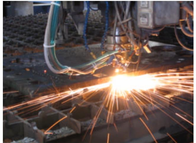
**Figures 50 & 51: LASOX System Installation in operation on Bender Shipbuilding's 6kW Tanaka Laser**
