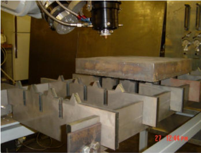
Figure 2: Fiber Laser Set Up With Thick Steel
