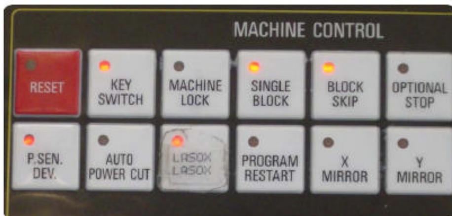
Figure 38: Photo of the LASOX key pad control button
