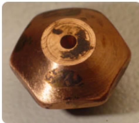
Figure 21: Copper nozzle with anti-spatter brushed off after a series of pierces
