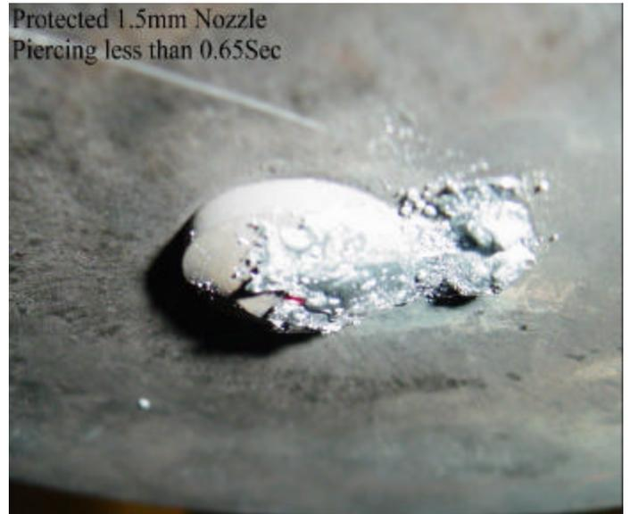
The graphite shield was able to prevent the adhesion of splatter to the copper nozzle, but the shield came off from the nozzle due to thermal expansion, there by preventing continuous piercing test. Even when the graphite shield was glued to the nozzle, due to thermal expansion, the shield came off and prevented continuous piercing experiments. The conclusion of the experiments led to the necessity of a new shield design with an improved holding mechanism for adhesion to the copper nozzle.
