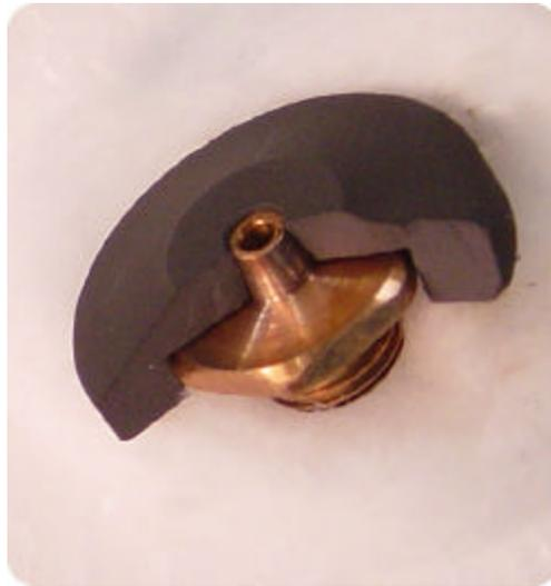
**Figure 6: Graphite Shield Cross-Section**
