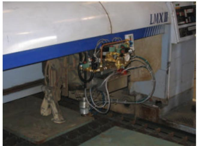
Figures 44 & 45: LASOX System Installation on Bender Shipbuilding's 6kW Tanaka Laser
