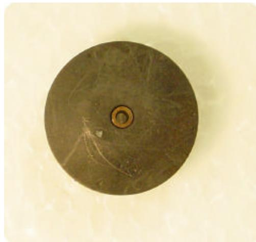
**Figure 5: Graphite Shield with Copper Tip**
