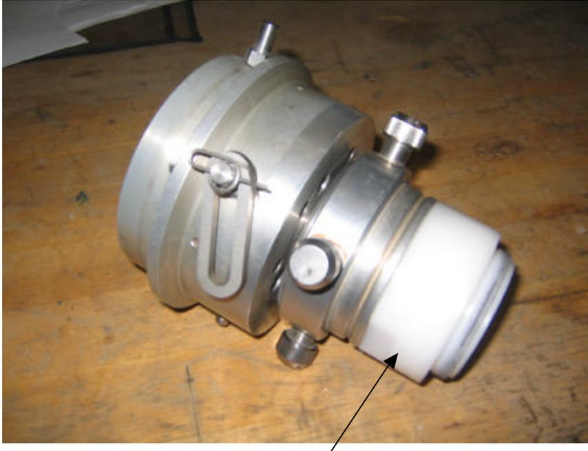
**Figure 42: Isolator attached to the LASOX head**
