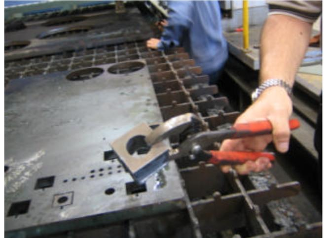
**Figure 48: Initial test pieces cut with LASOX**
