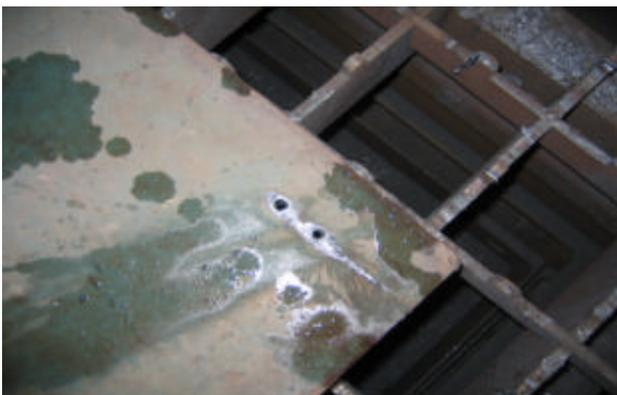
Figure 46: Initial test pierces made with LASOX
