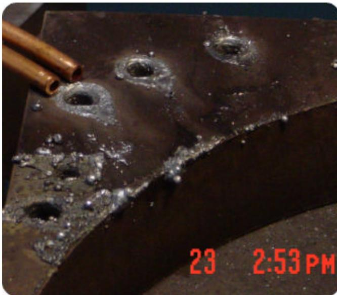
Figure 27: Quick Test #1 partial piercing holes
