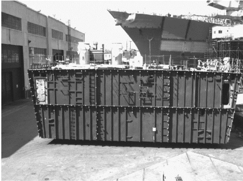
Figure 5b – Unit end measurements to determine unit make-up alignment accuracy
