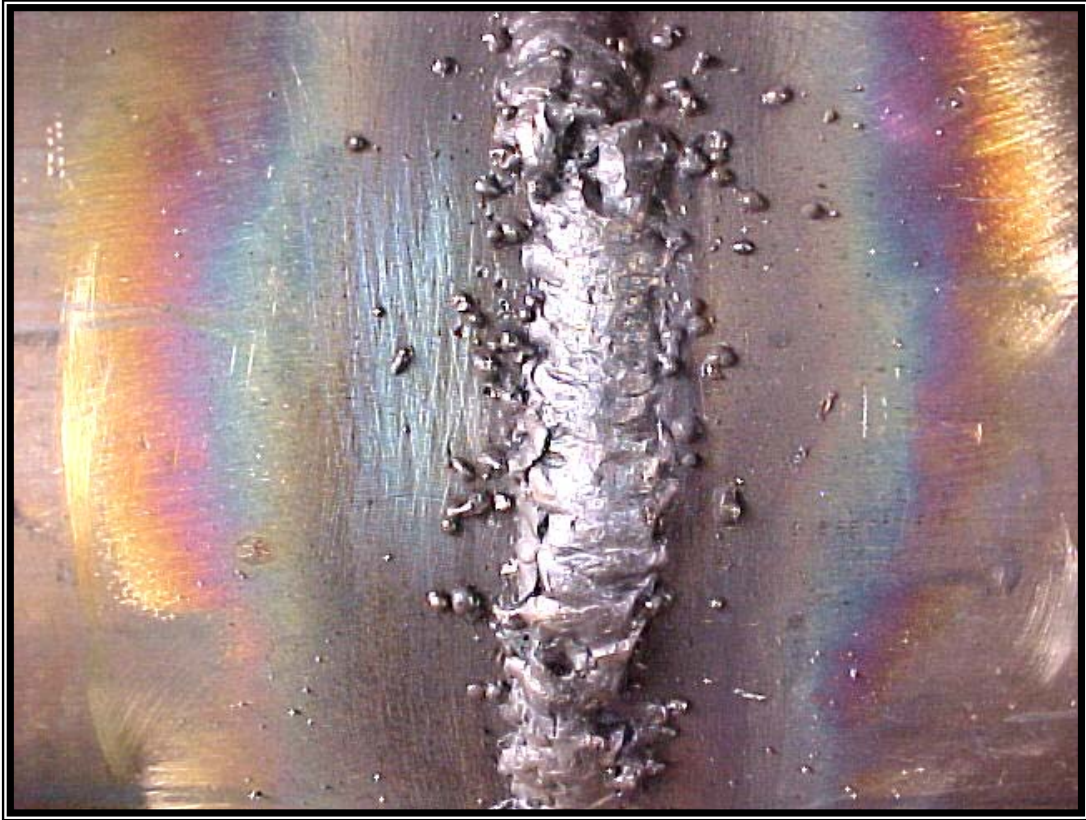
Figure 17 Cover pass starting at 2 o'clock to 1 o'clock on 6½ inch diameter x 1/8 inch wall CuNi 90/10 pipe with backing ring by FCAW using #A-6 electrode.
