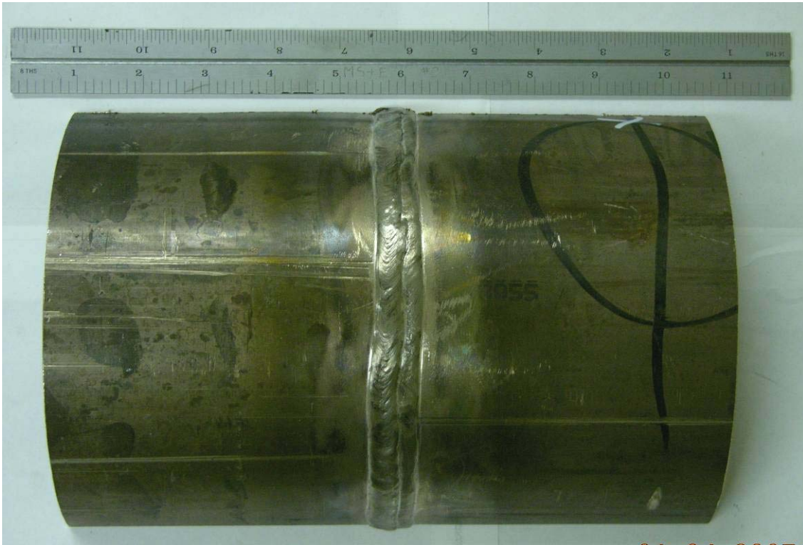
Figure 11 Current practice of GMAW-p of 6½ inch diameter x 1/8 inch wall CuNi 90/10 pipe using EN67 solid filler metal.
