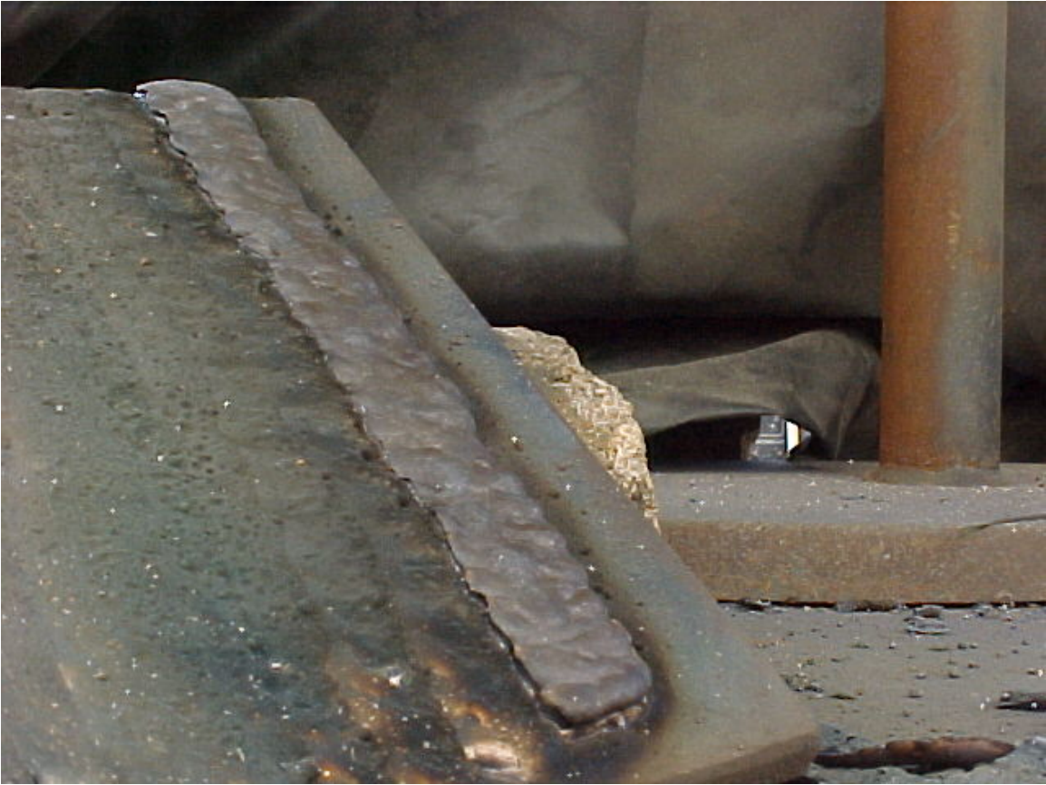
Figure 18 Bead-on-plate weld showing the excellent detachability of the A-6 electrode.
