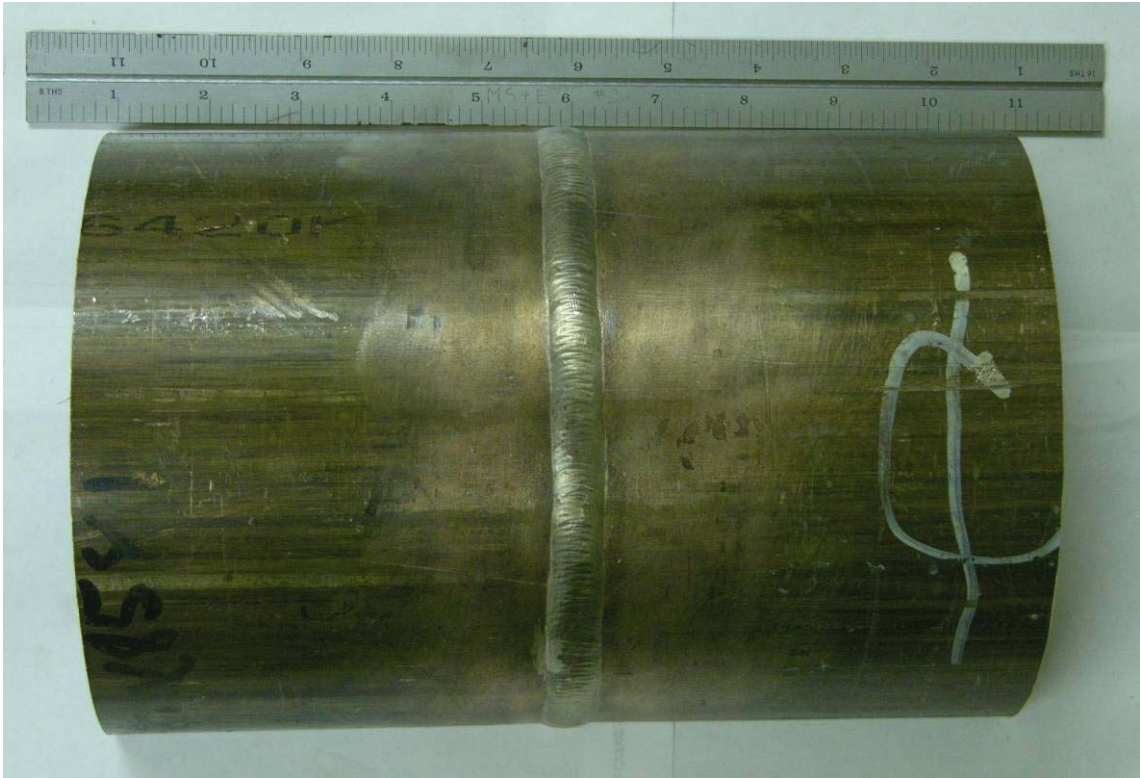
Figure 10 Current practice of GTAW of 6½ inch diameter x 1/8 inch wall CuNi 90/10 pipe using ER67 solid filler metal.
