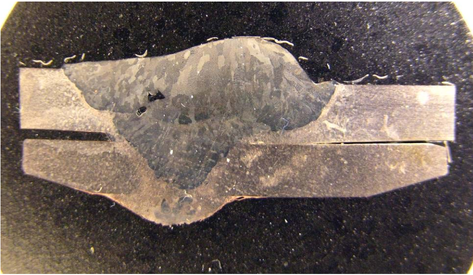
Figure 24 Metallographic section of test weld for operability using flux cored electrode #A-5 from Fabricator "A". Weld metal was deposited on 6½ inch diameter x 1/8 inch wall CuNi 90/10 pipe with backing ring by FCAW and C-25 shielding gas.
