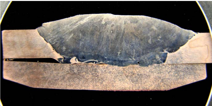
Figure 25 Metallographic section of test weld for operability using flux cored electrode #A-6 from Fabricator "A". Weld metal was deposited on 6½ inch diameter x 1/8 inch wall CuNi 90/10 pipe with backing ring by FCAW and C-25 shielding gas.
