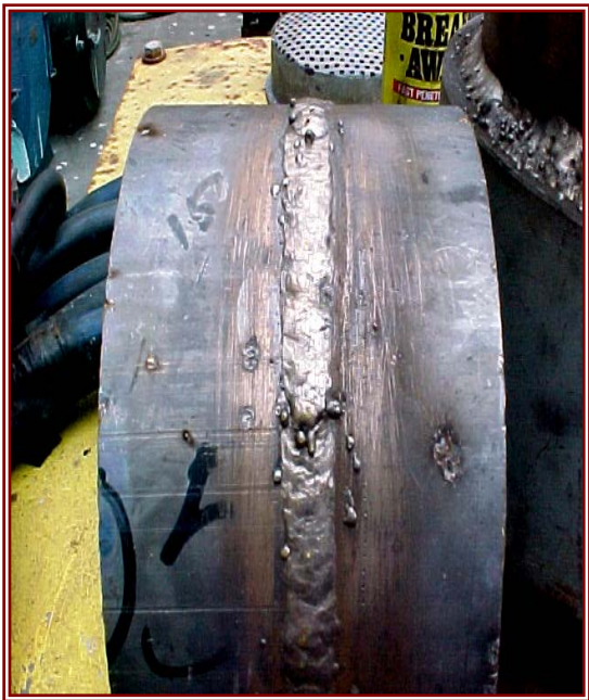
Figure 14 First test weld for operability performed at NASSCO using EN67T-1 flux cored electrode #A-3 from Fabricator "A". Weld metal was deposited on 6½ inch diameter x 1/8 inch wall CuNi 90/10 pipe with backing ring by FCAW. Top photo: out-of-position welding starting overhead 6 to 4 o'clock; Bottom photo: flat position welding.
