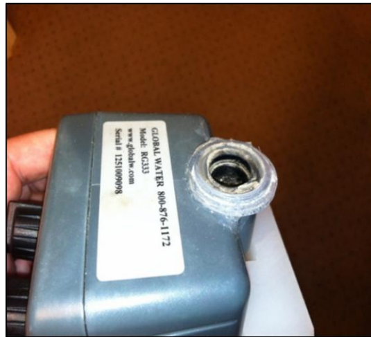
Figure 26. Faulty seal on Rain Gauge
