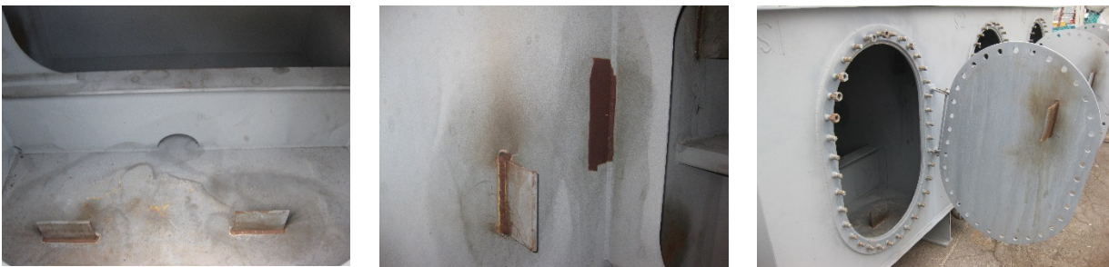
Figure 1. Representative pictures of weathered pre-construction primer in the simulated ballast tanks.
