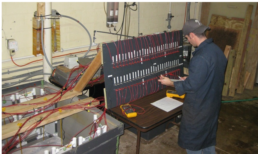
Figure 2. Cathodic disbondment test arrangement.
