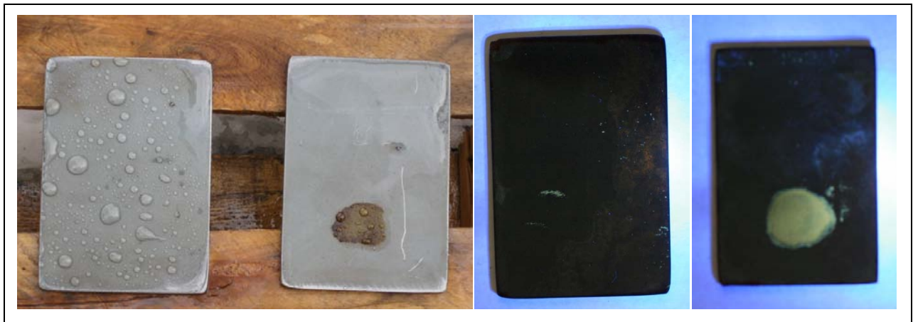
Figure 9. Representative Test panels after Hose Washing.
