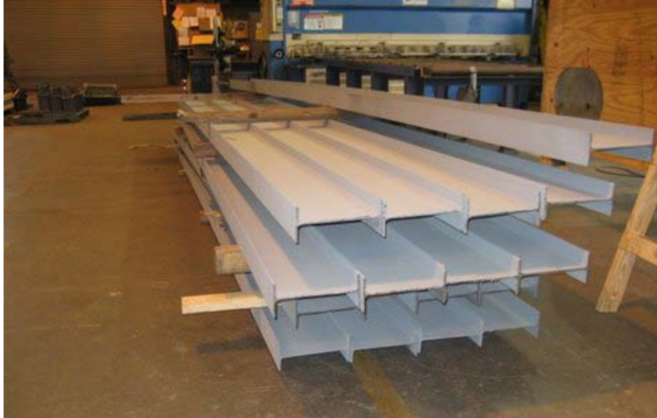
Figure 1. Shapes after being primed with 0.7 mils of PCP.
