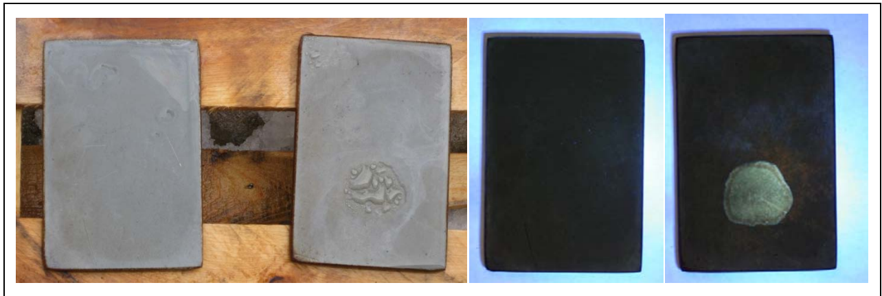
Figure 8. Representative Test Panels after 2500 psi pressure wash.
