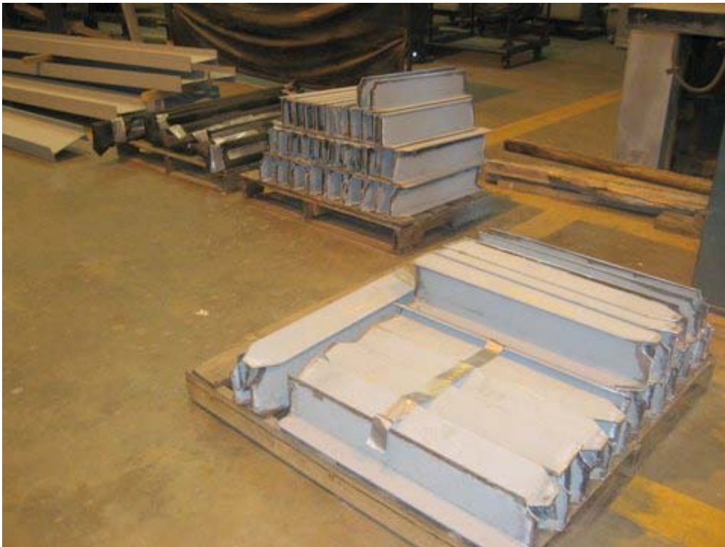
Figure 2. Stiffeners cut to fit from the primed shapes.
