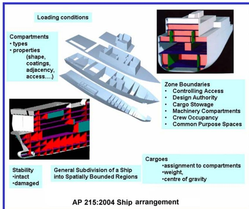
**FIGURE 4 – ISO 10303-215 Ship arrangement**
