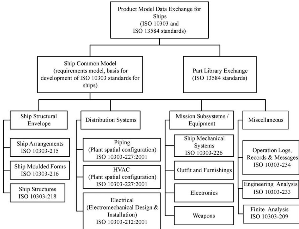
**FIGURE 2 – The ISO STEP Shipbuilding Standards**
