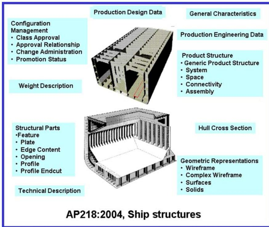
**FIGURE 9 – ISO 10303-218 Ship structures**
