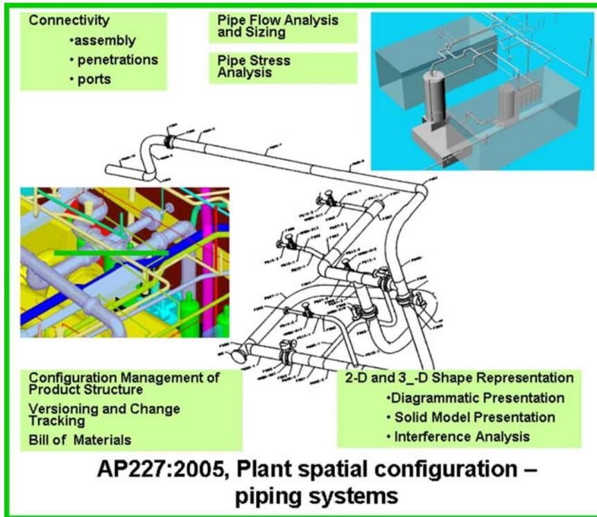
FIGURE 5 – ISO 10303-227 Plant spatial configuration – Piping
