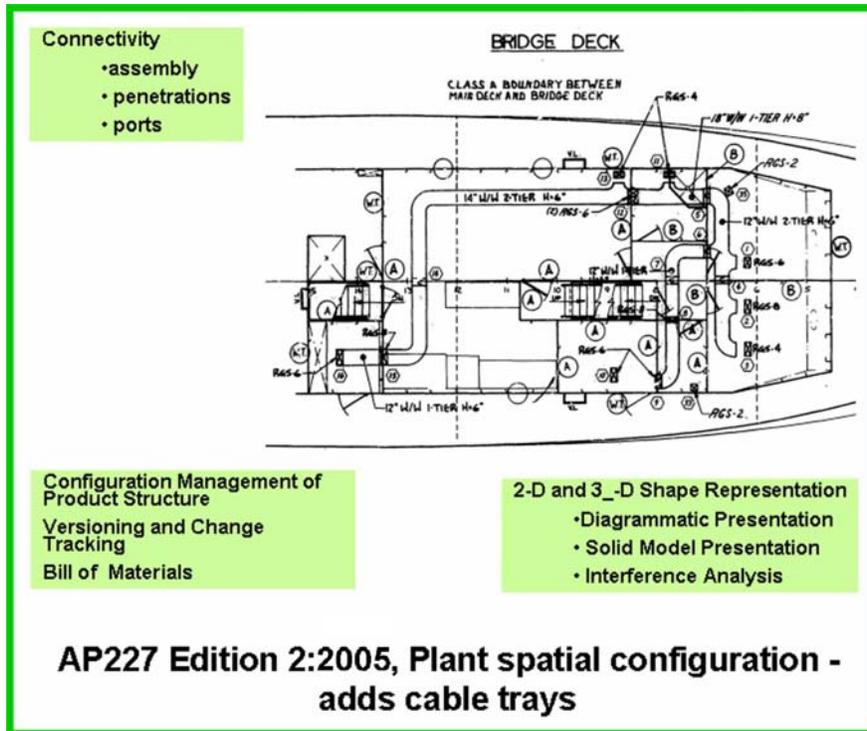
FIGURE 7 – ISO 10303-227 Plant spatial configuration – Cable trays
