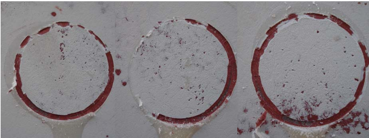
Close-up of adhesion tests at test location 2.
