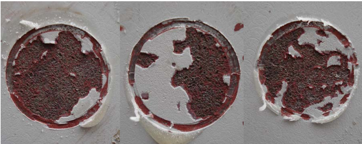
Close-up of adhesion tests at test location 7.
