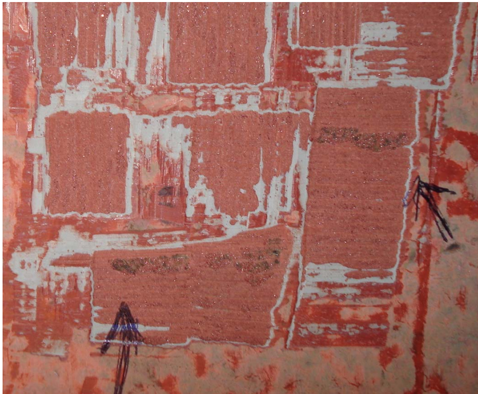
Figure 7. Small areas of substrate revealed when excavating at test location 8.
