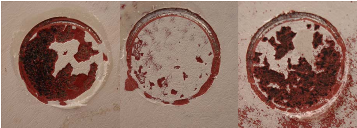
Close-up of adhesion tests at test location 3.
