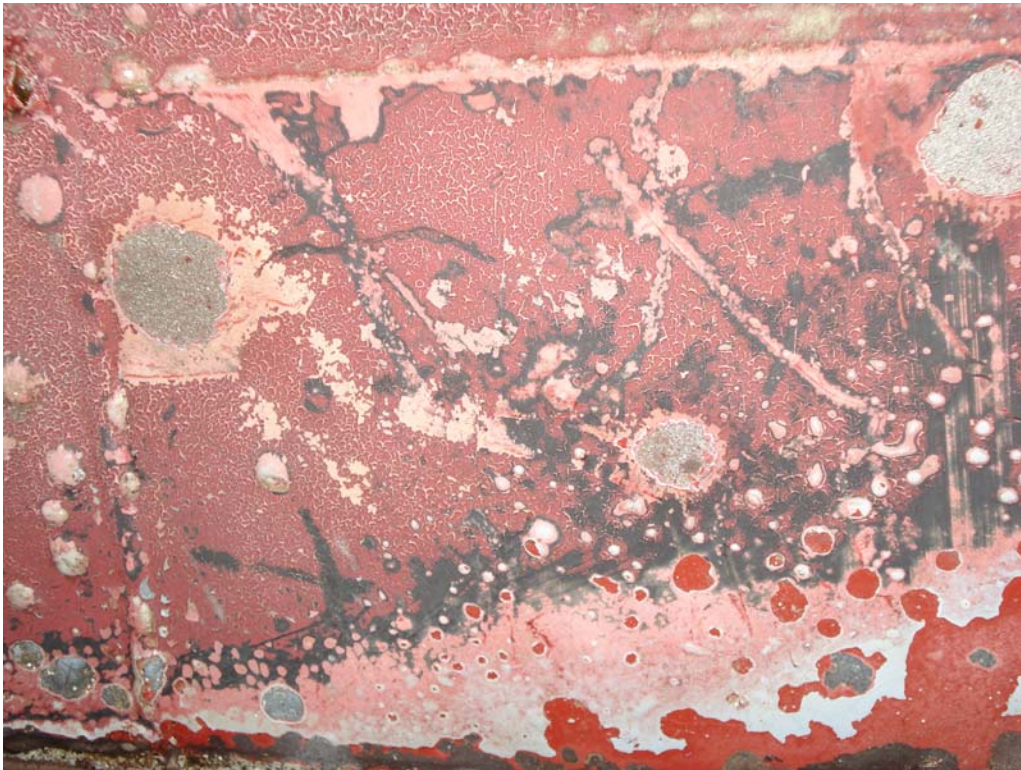
Figure 5. Representative blistering along the keel in the vicinity of the stern air masker.
