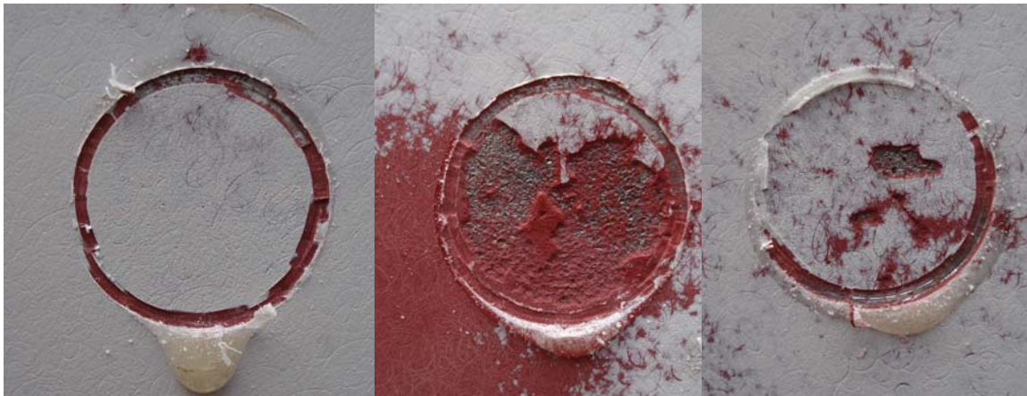
Close-up of adhesion tests at test location 4.
