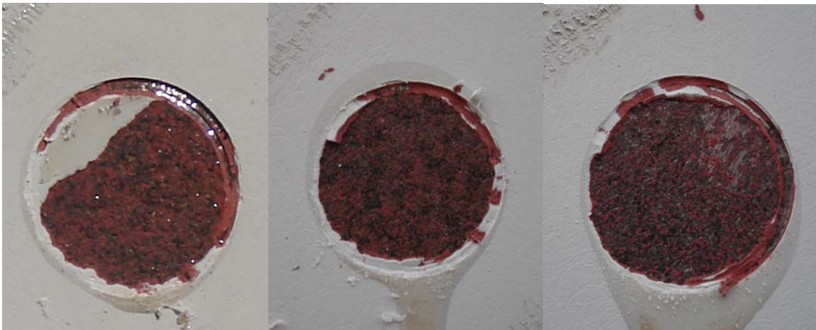
Close-up of adhesion tests at test location 1.
