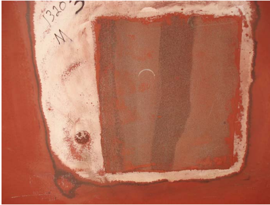
Figure 8. Test Patch 3 with nominally 100 square inches of coating removed.
