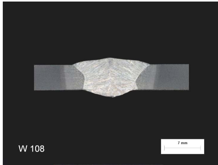
Figure 20 - Weld Made with Preferred 5-mm Plate Procedures (W108)
