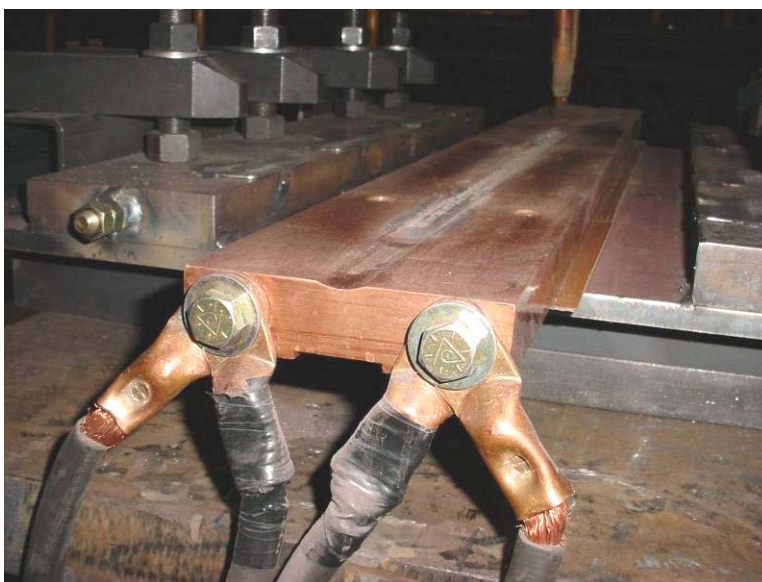
Figure 10 - Electrical Grounding Arrangement on Improved FCB Bar
