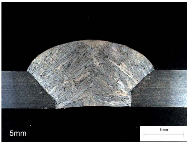
Figure 5 - Modified S-SAW Weld 5-mm Plate
