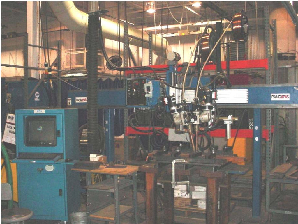
Figure 12 - Tandem SAW Work Area at EWI
