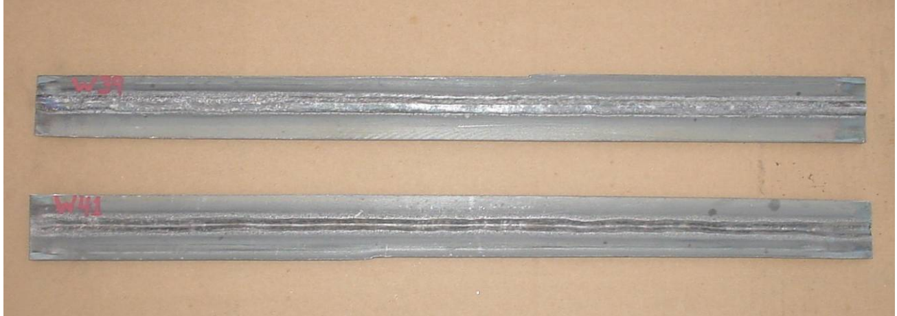
Figure 15 - Inconsistent Suck-Back Defects on Welds Made with Identical Parameters
