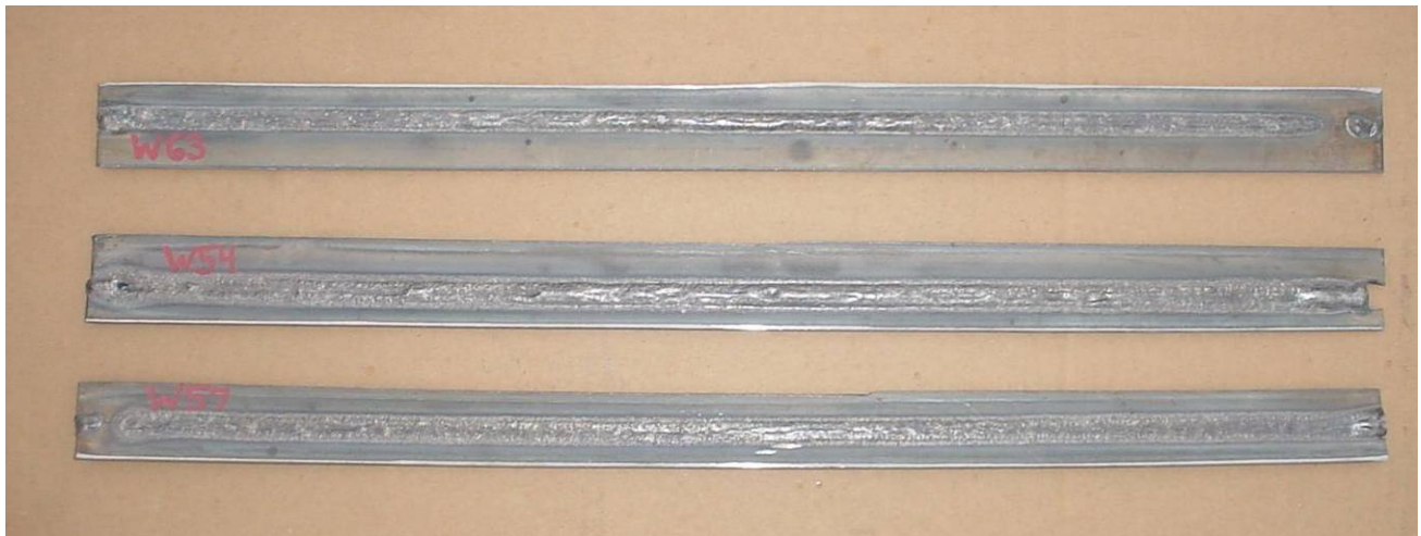
Figure 16 - Welds with Pronounced Suck-Back in the Middle Span
