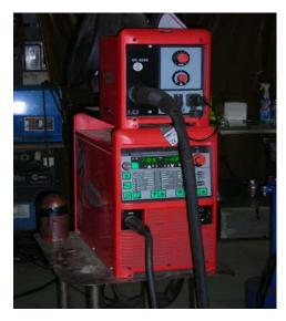
Fronius Transpulse Synergic 3200 power supply and Feeder
