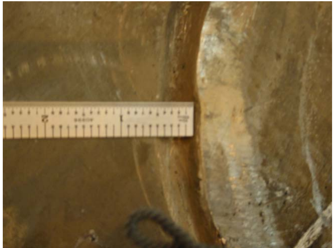
Example shown of a back gouge of \frac{1}{2} " (12 mm) 154
