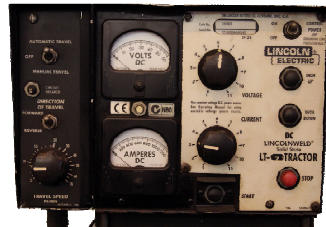
Lincoln Electric LT-7 Tractor Control Box
