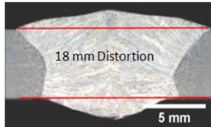
Conventional Single-Sided Tandem SAW
