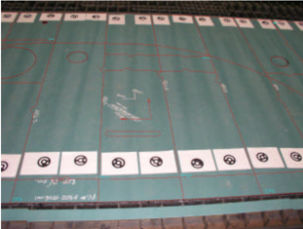
Figure 49: Digital photo with autotargets and AutoCAD model/drawing overlaid (red lines).
