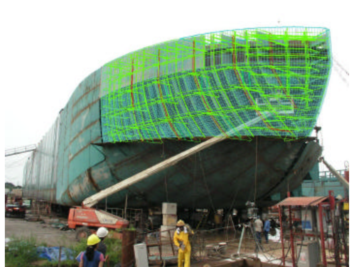
Figure 52 & 53: Generated 3D Hull Shape (red lines) & New model hull shape overlaid.
