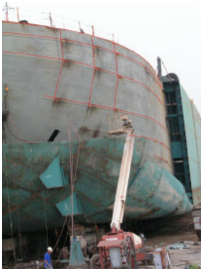
Figure 52 & 53: Generated 3D Hull Shape (red lines) & New model hull shape overlaid.
