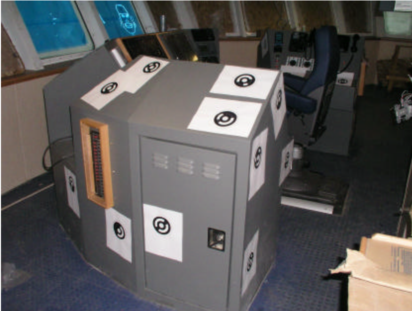
Figure 56: Photo of console with autotargets
