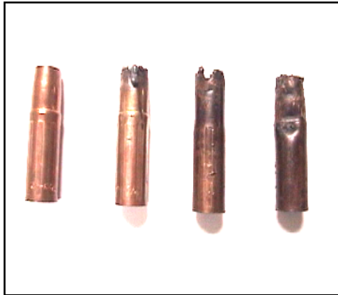
Figure 1 - New Nozzle, Slag Damage, Arc damage, Plier Damage
