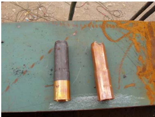
Figure 15 Blackjack & Standard Nozzles After Use - Arc Damage on Right
