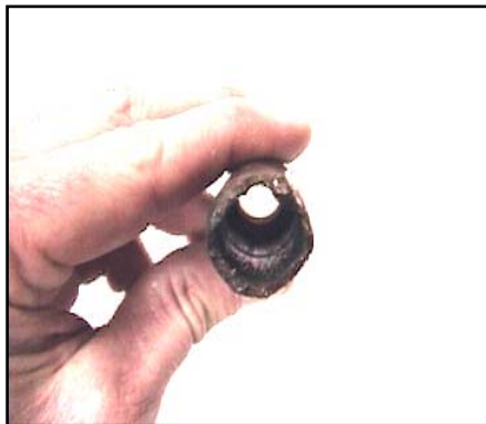
Figure 5 - Arc Damage Inside
