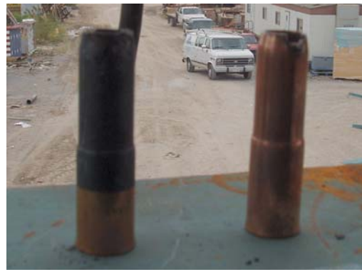
Figure 14 Blackjack & standard nozzles
