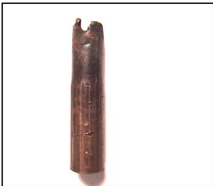
Figure 4 - Nozzle Arc Damage
