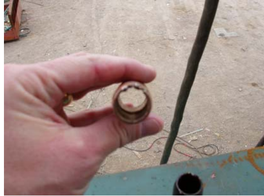
Figure 16 Inside Damaged Standard Nozzle
