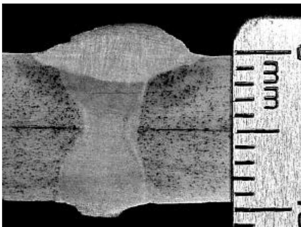
Figure 7: Cross-section of Bead-on-plate Weld Obtained Using Stationary Bar. Material: DH 36, Thickness: 3/8 in, Position: Vertical-down, Welding Speed: 150 mm/minute (6 in./min), Welding Current: 160 A. The cover pass was done using GMAW.
