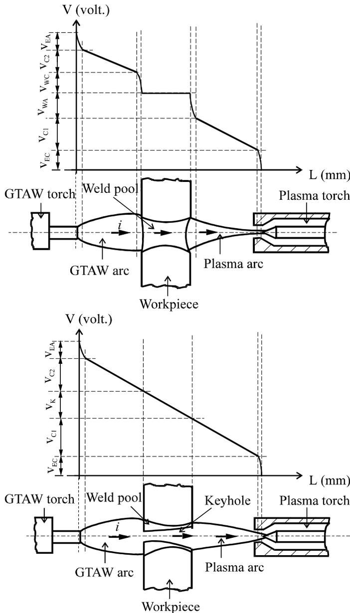
Figure 3: Voltage Decomposition in DSAW.
