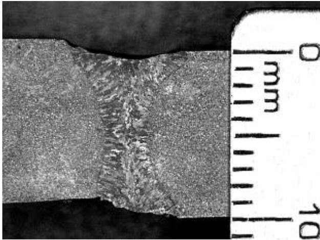
Figure 4: Butt Weld Made Using Controlled Pulse Keyhole DSAW Process. Thickness: 10 mm, Material: DH36, Welding position: vertical-down, Filler metal: none, Travel speed: 120 mm/minute, peak current: 140 A, base current 80 A.
