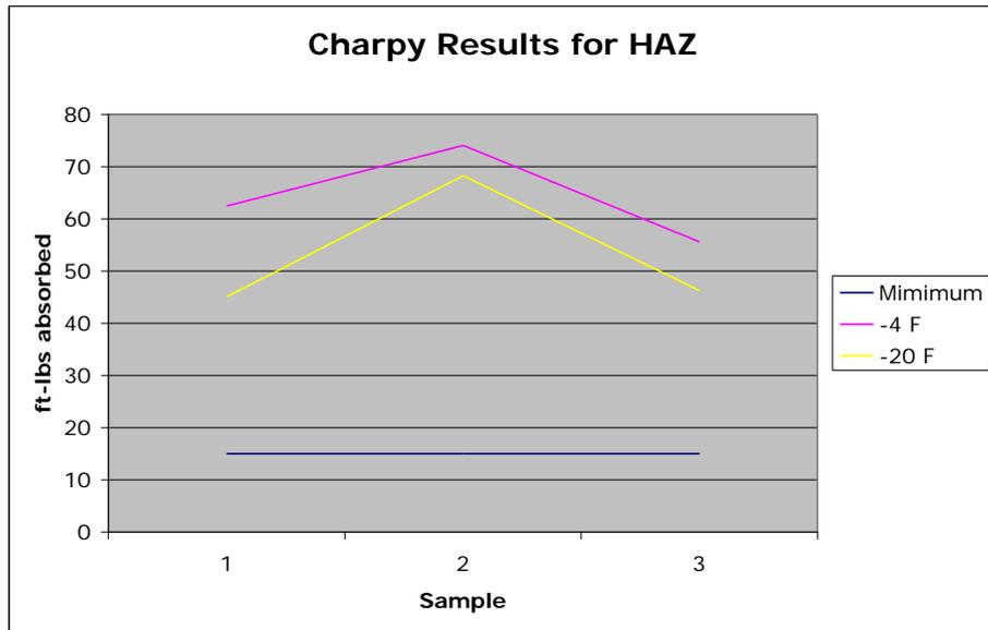
Figure 12: Toughness Values for HAZ of the DSAW Samples Using INCONEL® 625 Filler metal. All test coupons were ¾ sub-sized and the results were converted per SAE J1194.
