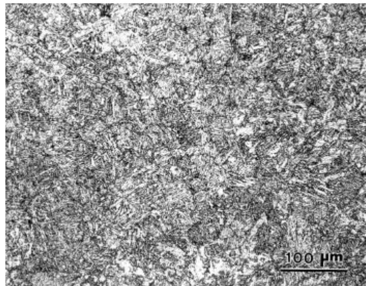
(C) DSAW Weld Metal with ER-70S filler metal
