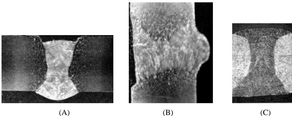
Figure 9: Cross-section of Double-sided Arc Welds on 3/8 in. DH36. (A) Flat position; (B) Horizontal position; (C) Vertical—down position with pre-deposited filler metal.
