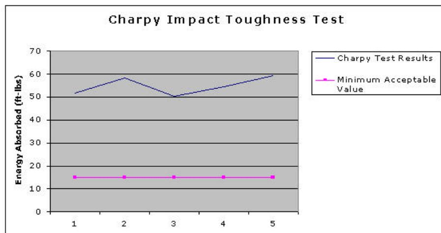
Figure 11: Toughness Values for DSAW Samples Using INCONEL® 625 Filler Metal.
