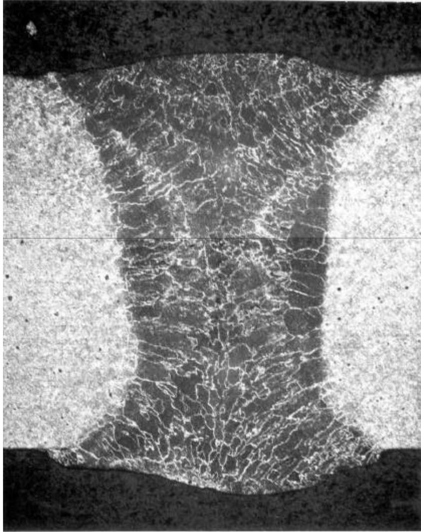
Figure 10: Cross-section of 3/8" DH36 with 0.06" Gap and ER-70S Filler Metal.
