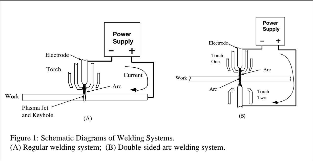
Figure 1: Schematic Diagrams of Welding Systems.
