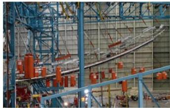
Mitsubishi Heavy Industries (MHI) is using Aurora to accelerate its production of Boeing 787 Composite Wing Boxes.
