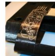
UAV wing with strain sensor
