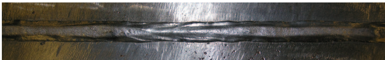
Figure 3.26: 1” DH36 One-sided Weld, ESAB OK10.62 – Root Side
