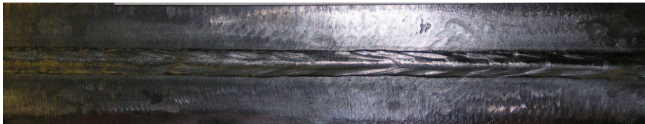
Figure 3.31: 1" HSLA-65 One-sided Weld, Lincoln MIL800-H – Root Side
