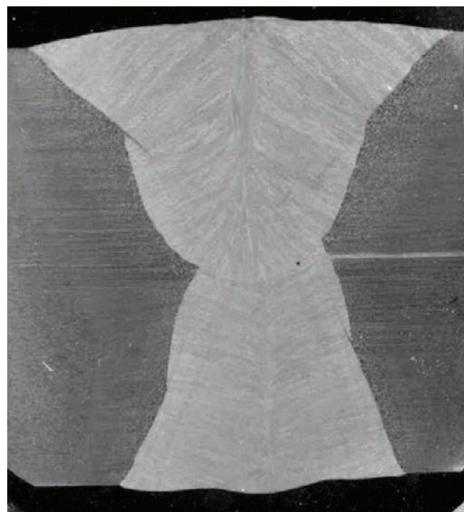
Figure 3.35: HSLA-65 OSW with 5/32" Root Gap (2.5X Mag)
