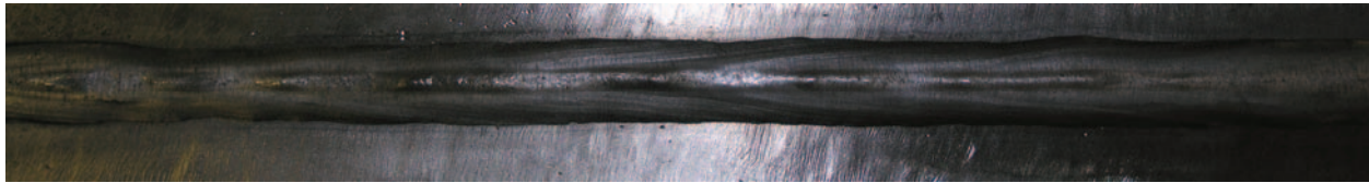
Figure 3.25: 1” DH36 One-sided Weld, ESAB OK10.62 – Cap Side
