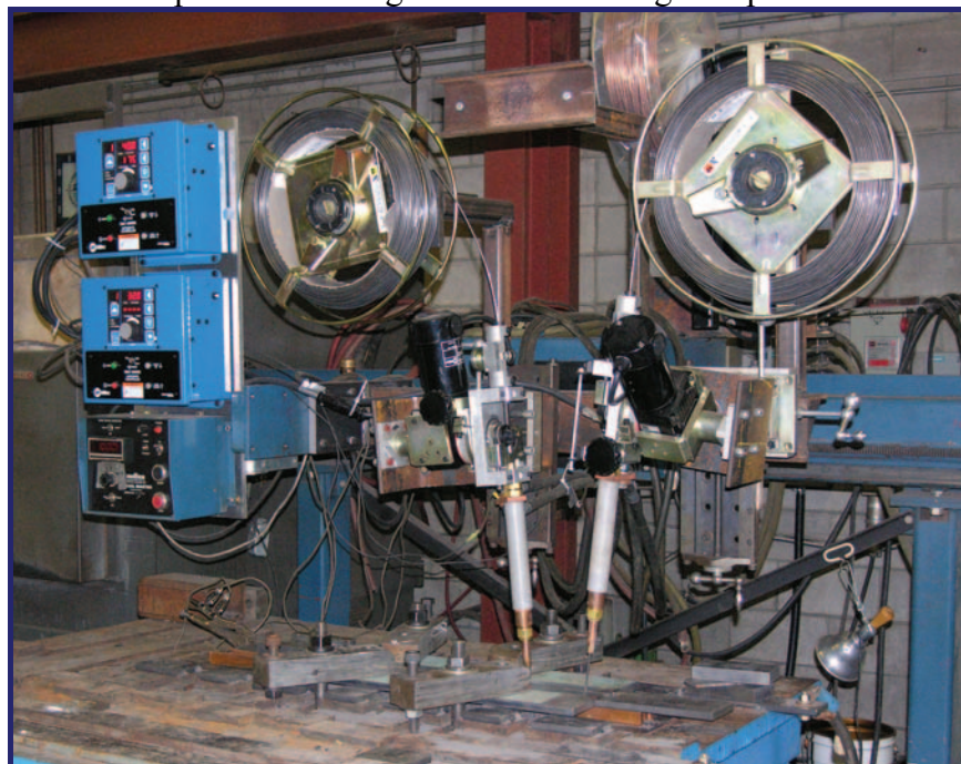
Figure 3.16: Set-up for Tandem One-sided Welding
