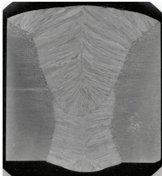
Figure 3.33: 1” HSLA-65 One-sided Weld, Lincoln MIL800-H – Macro – 2.5X Mag
