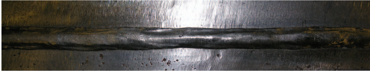
Figure 3.29: 1" HSLA-65 One-sided Weld, ESAB OK10.62 – Root Side
