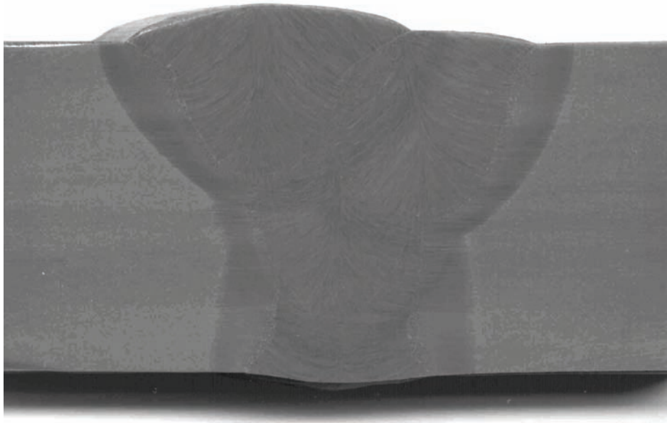
Figure 3.30: 1” HSLA-100 Tandem OSW – Four Passes
