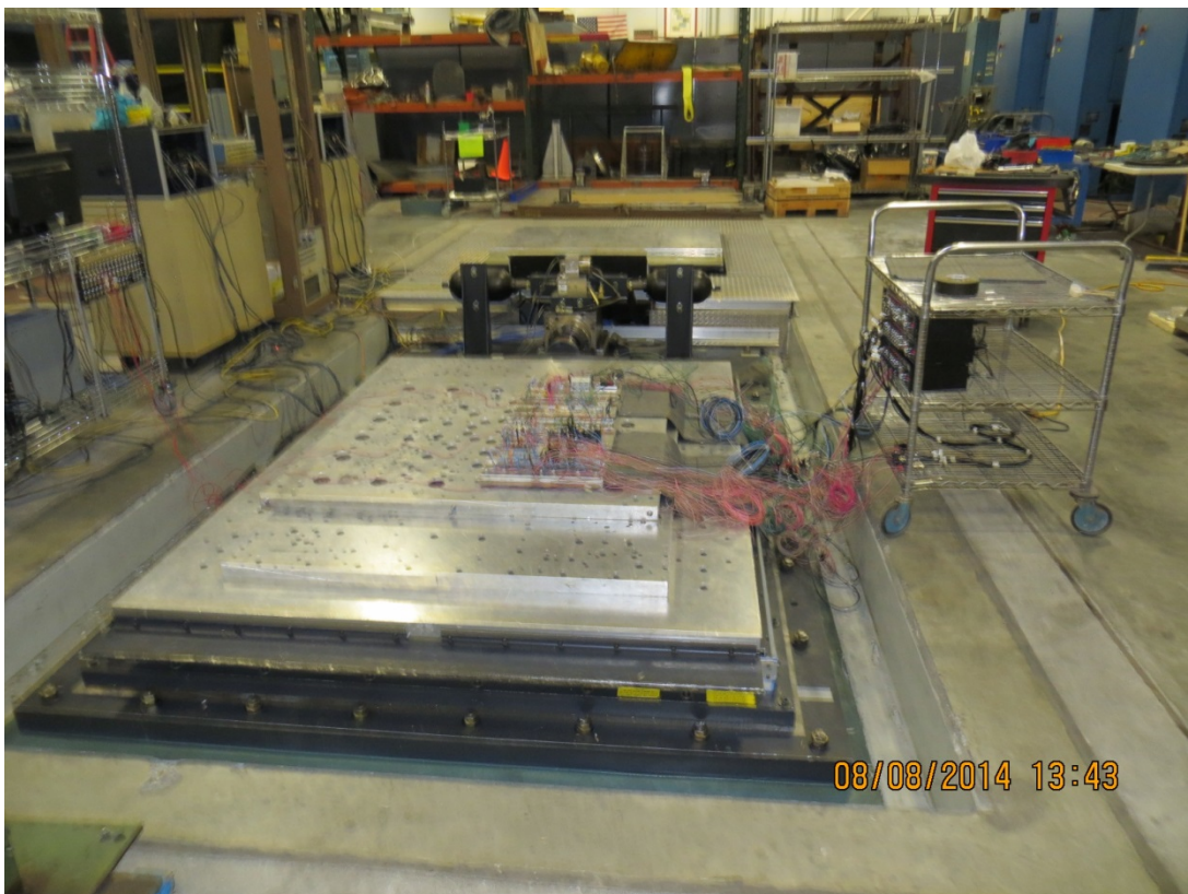
Photo 4 – File No. FB14-0563 Vibration test setup in the up/down axis
