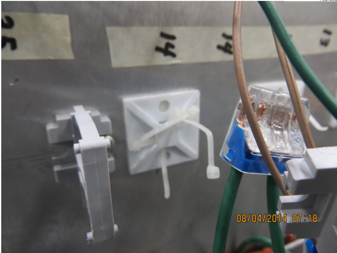
Photo 29 – File No. JP14-0168 View showing connector #14 with broken ties after Shock Blow No. 3
