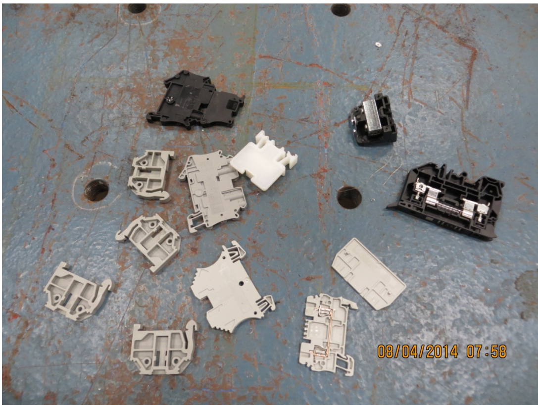
Photo 40 – File No. JP14-0179 View showing dislodged connector pieces after Shock Blow No. 3
