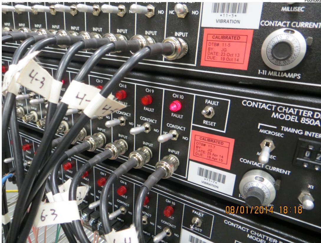
Photo 7 – File No. AG14-1038 View after Shock Blow No. 1 in the back direction, item #24 had chatter
