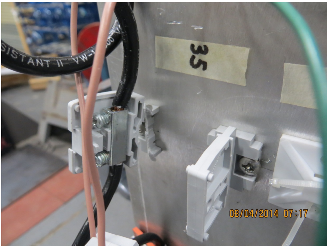
Photo 28 – File No. JP14-0167 View showing connector #35 broken at base after Shock Blow No. 3
