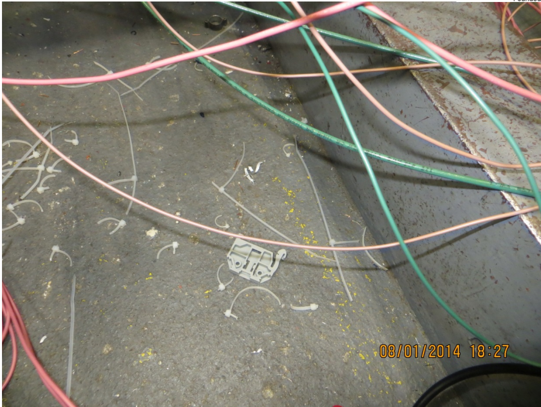
Photo 11 – File No. AG14-1042 View after Shock Blow No. 2 in the back direction, parts fell off and others were loose
