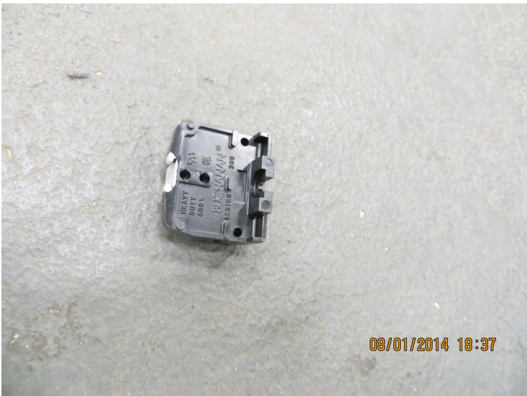
Photo 22 – File No. AG14-1053 View after Shock Blow No. 3 in the back direction, parts flew off and came loose
