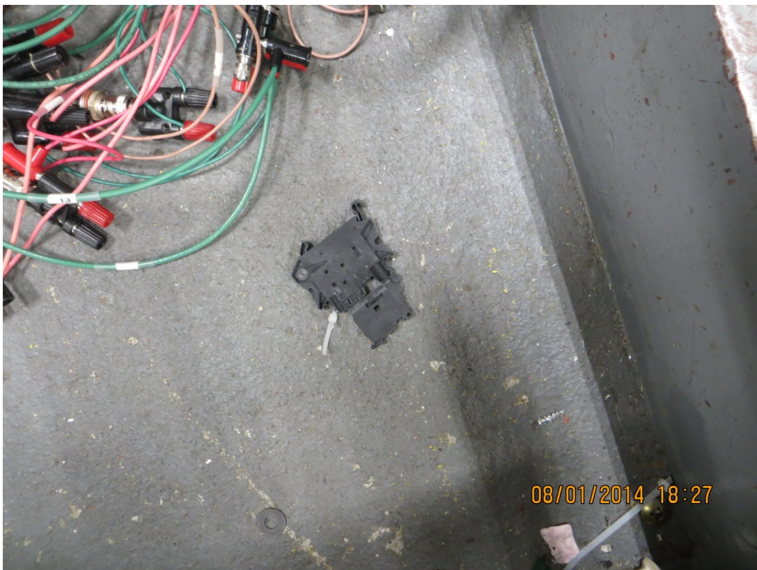
Photo 12 – File No. AG14-1043 View after Shock Blow No. 2 in the back direction, parts fell off and others were loose
