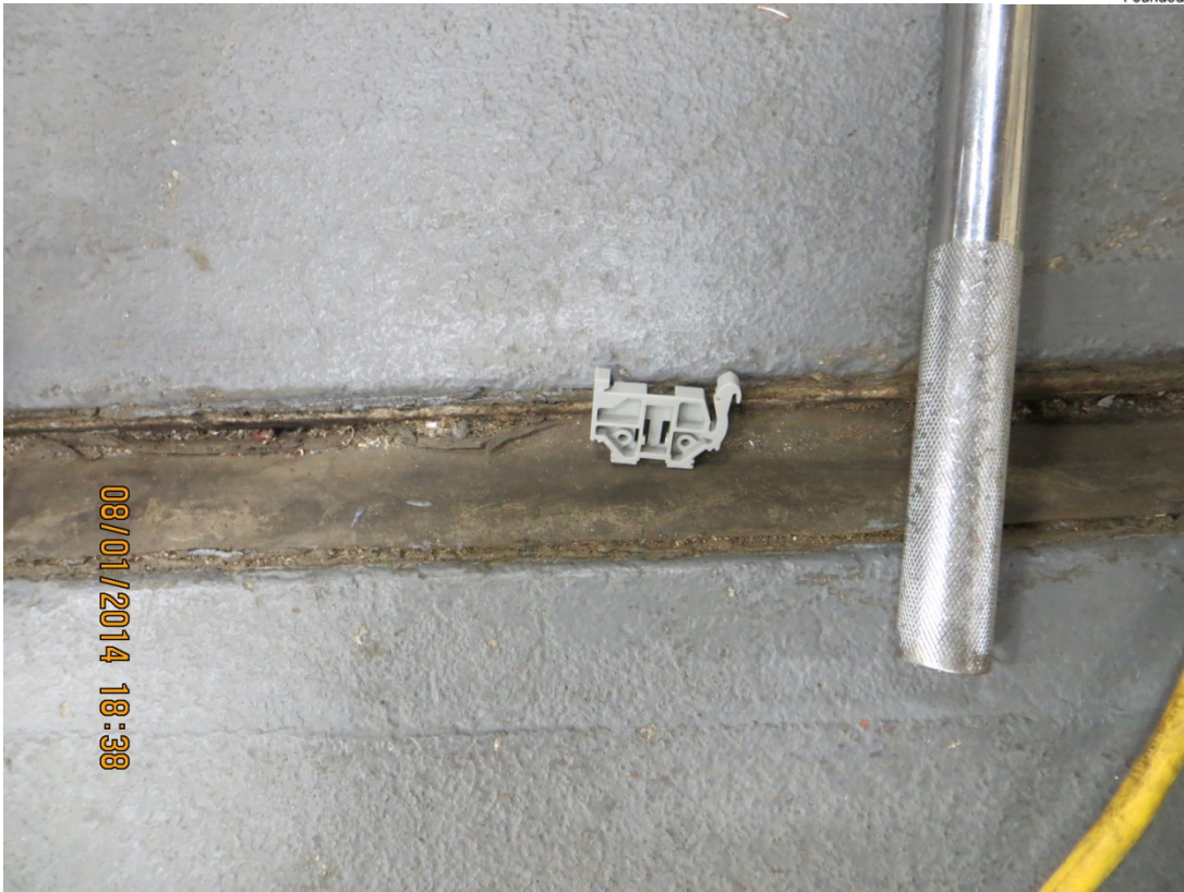
Photo 23 – File No. AG14-1054 View after Shock Blow No. 3 in the back direction, parts flew off and came loose
