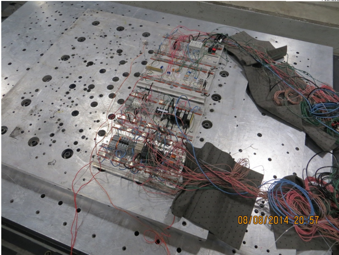
Photo 7 – File No. FB14-0567 Vibration test setup in the side/side axis for exploratory
