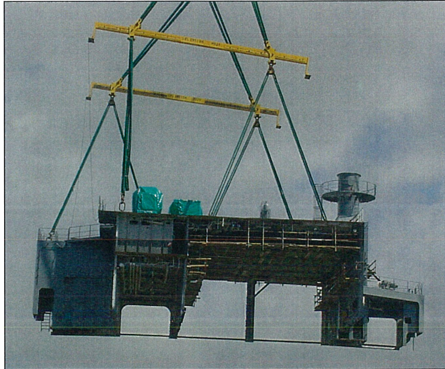
Figure 3 – Ship Block Lift with Extra Structure For Lift
