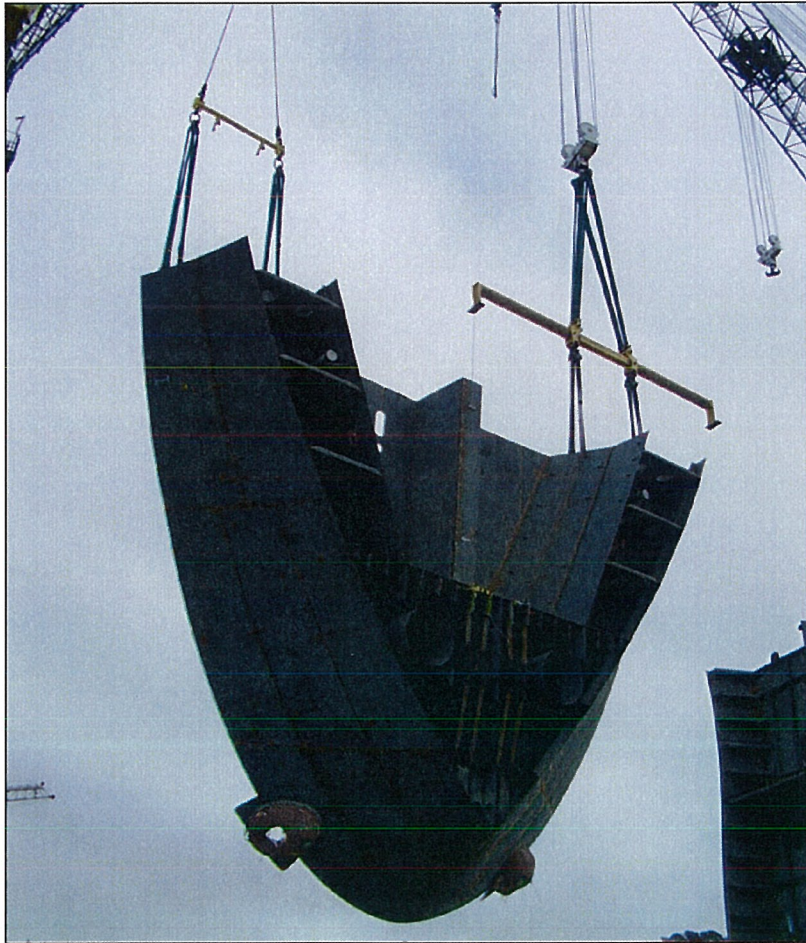
Figure 4 – Large Ship Bow Block Halfway Through Turn Operation
