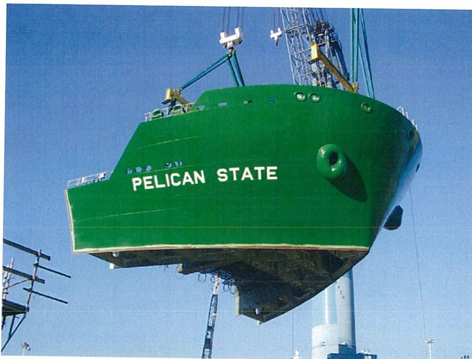
Figure 18: Lift of bow block using synthetic sling
