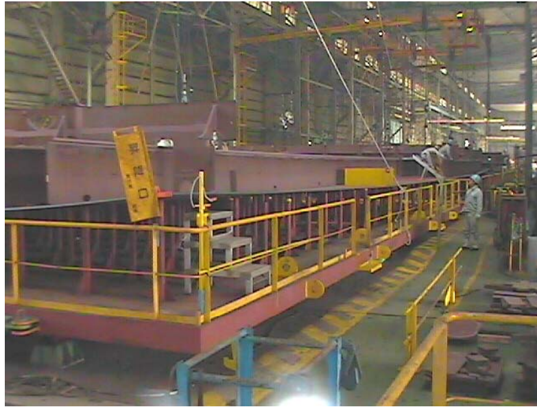
Photo 4: Curved Block Moving Process Line
