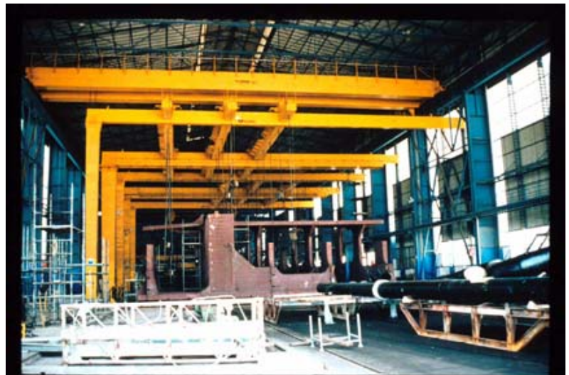
Photo 20: Welding Units Suspended from Overhead
