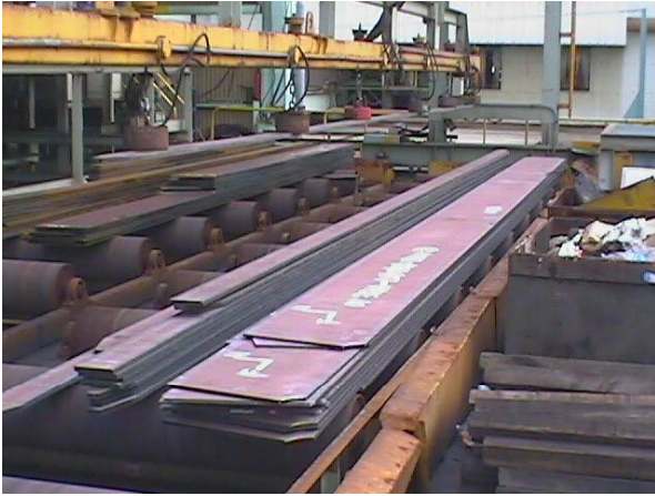
Photo 21: Sequenced Material for Profile Construction
