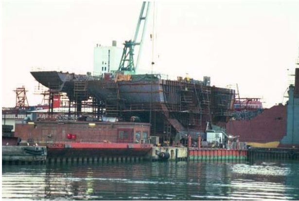
Photo 30: Turn-key Outfitting of Stern
