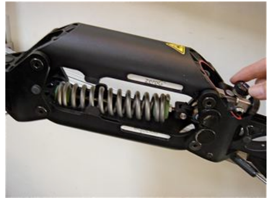
Figure 8 Link in position to adjust lift
