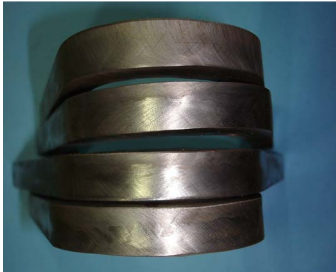
Figure 4.10: Side Bend Tests, 65-DS-1/2
