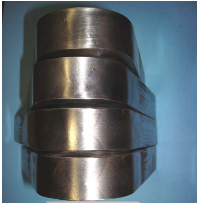
Figure 4.14: Side Bend Tests, 36-DS-1
