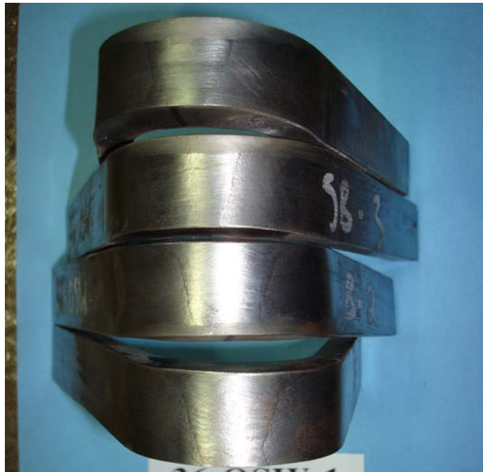
Figure 4.12: Side Bend Tests, 36-OSW-1
