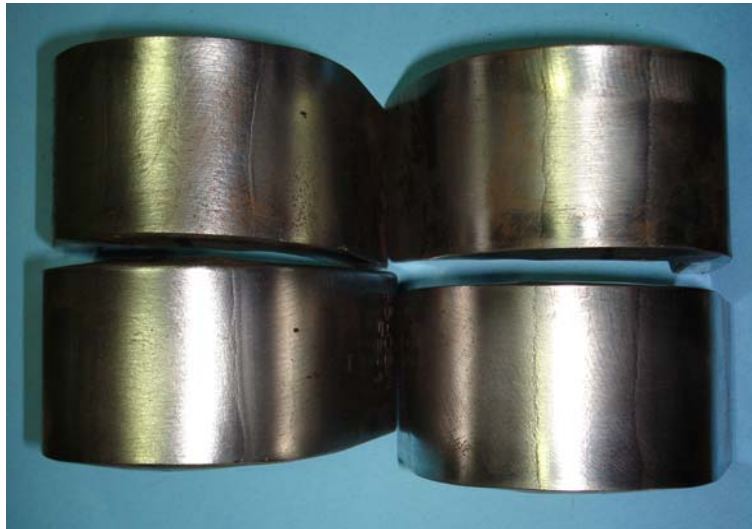
Figure 4.8: Face and Root Bend Tests, 36-OSW-1/2
