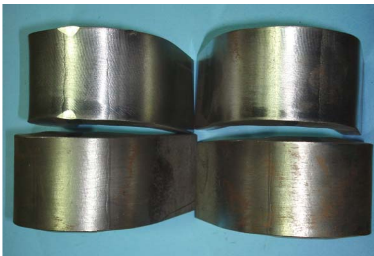
Figure 4.9: Face and Root Bend Tests, 65-OSW-1/2
