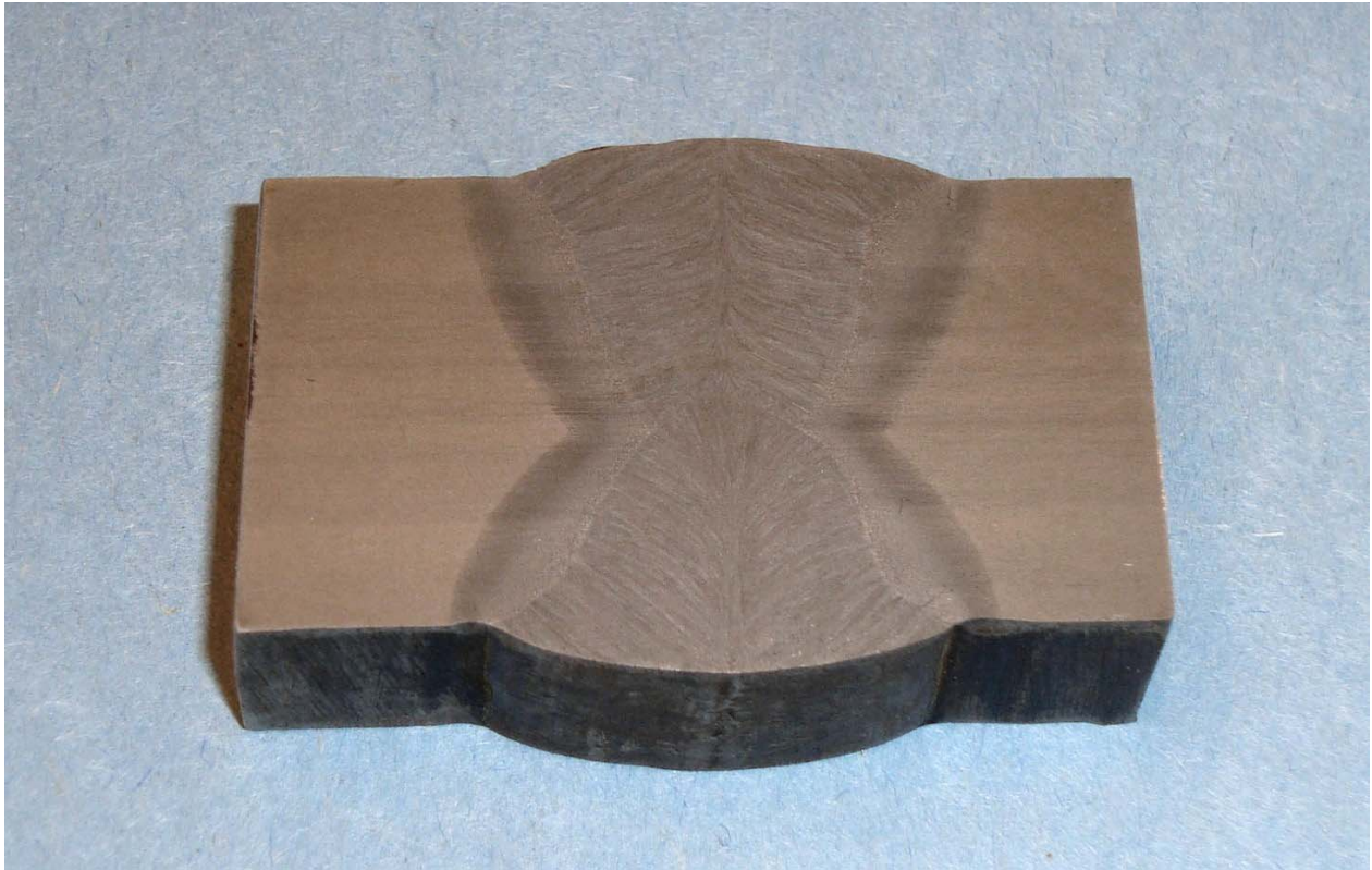
Figure 4.7: Sample Macro, 1" DS Weld Procedure
