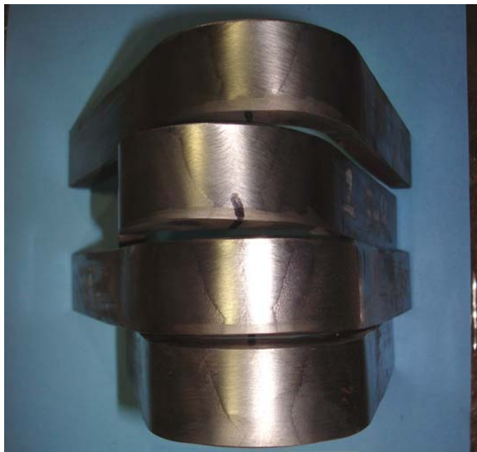
Figure 4.13: Side Bend Tests, 65-OSW-1
