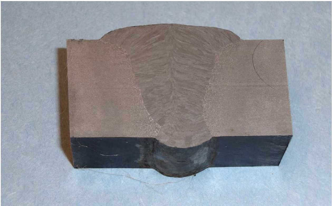
Figure 4.6: Sample Macro, 1" OS Weld Procedure
