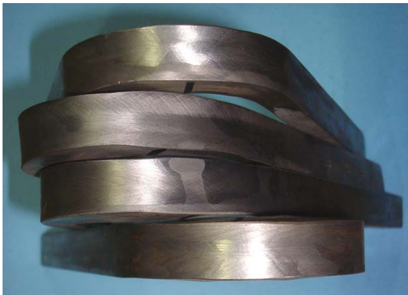
Figure 4.11: Side Bend Tests, 36-DS-1/2
