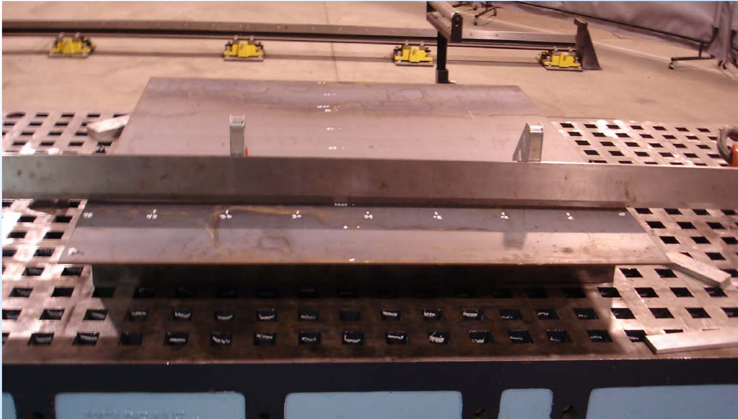
Panel after welding, set up for longitudinal distortion measurements.
