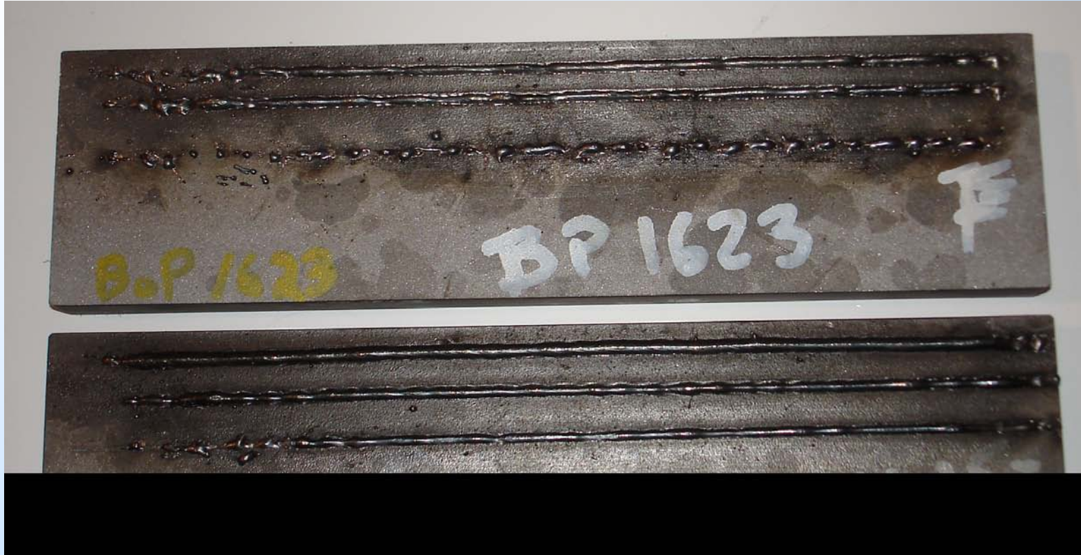
Top: GMAW-only; Bottom: Laser-Stabilized GMAW
