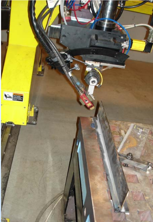
Left, Tee section set up for PCW tests. Right, welding underway. Red box in lead of the process is laser-seam tracker. Welding is GMAW only, welding speed: 40 ipm.
