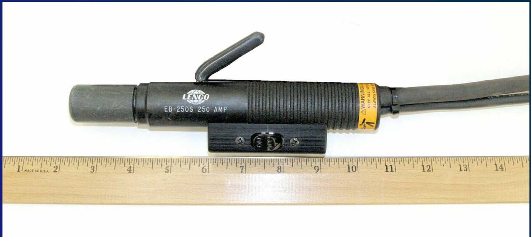
Lenco – based SMAW Stinger With Contactor Switch
