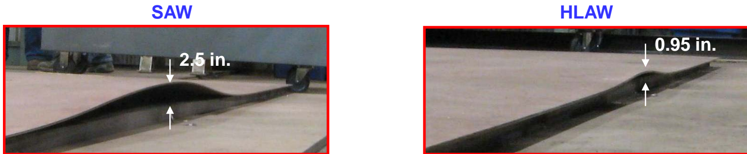
Distortion in 16x20 foot thin-steel panels welded using current shipyard practice (top) and hybrid (bottom) at BIW in January 2008. Overall, the hybrid welded panel was 4-times flatter than the conventional submerged arc welded panel
