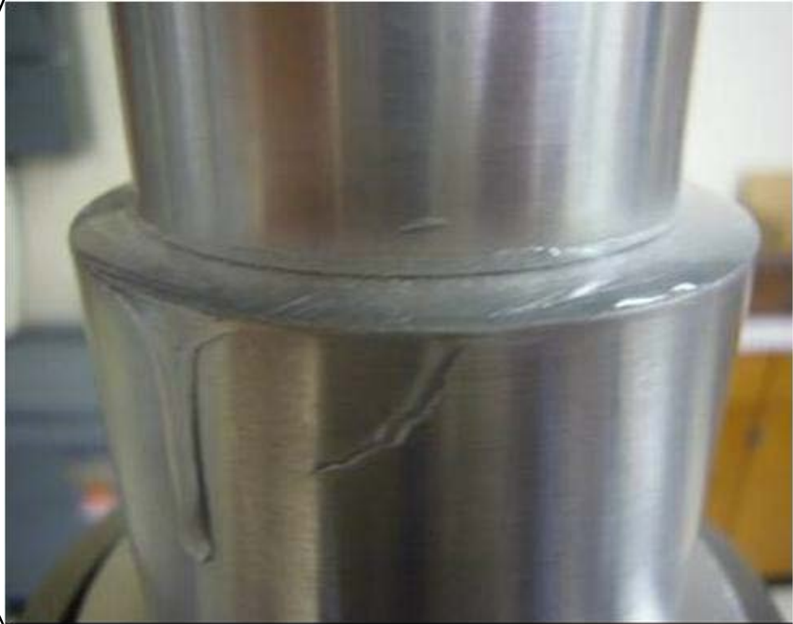
Attachment Blocks Bonded with Acrylic
