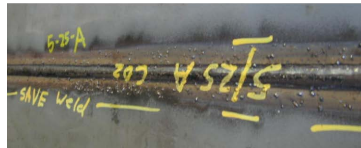
Figure 5 May 11 and May 25 Fiber Tape Backing on top of Copper Backing Bar, CO 2 Gas.
