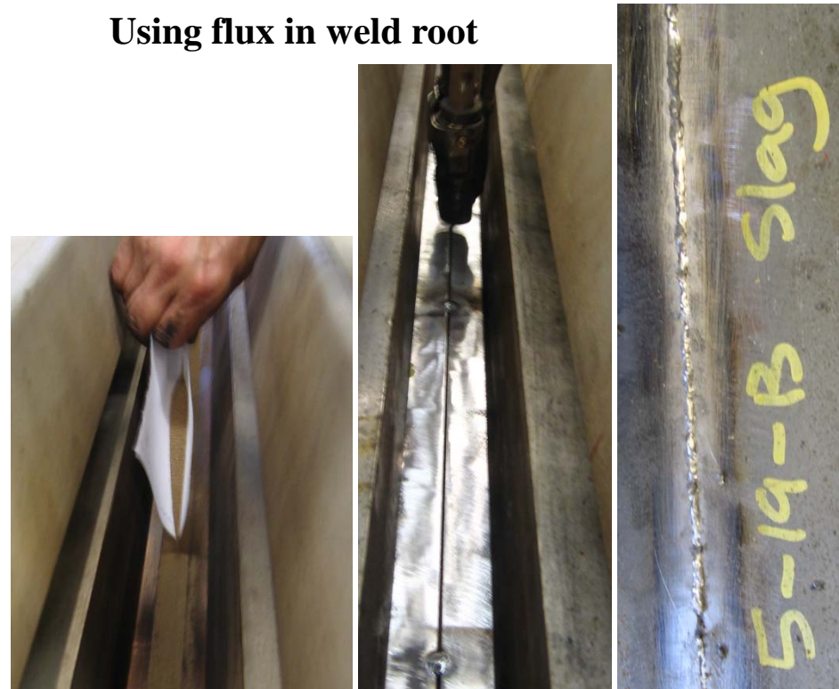
Figure 2 Test of May 19 with 3/32 Root Opening, Flux Root
