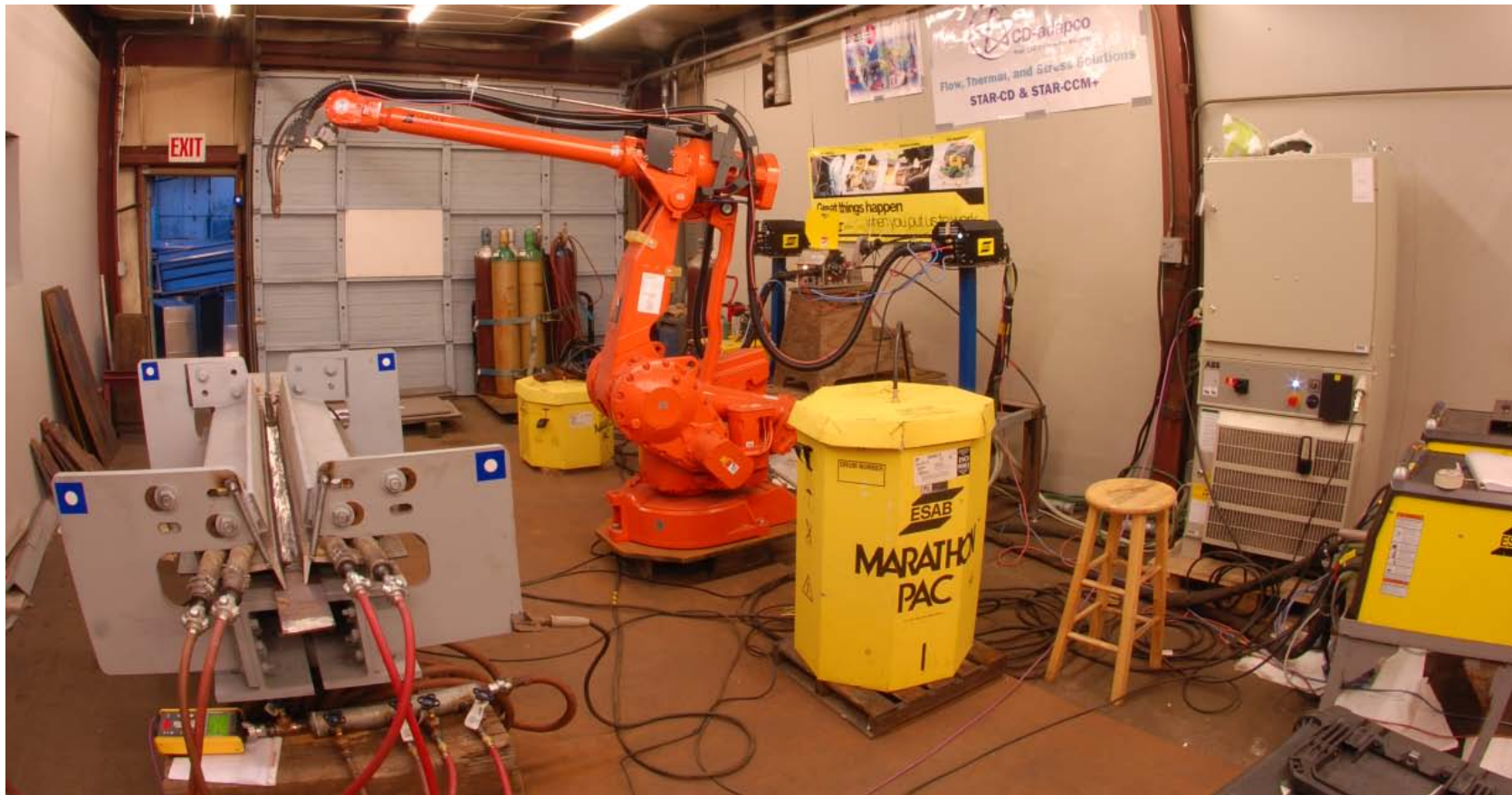
Weld Lab at Todd Pacific Shipyard with Weld Cell and Fixture
