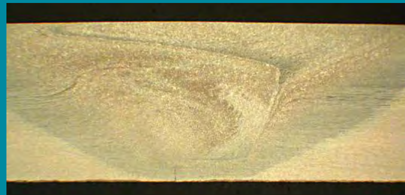
Defect free HSLA-65 FSW
