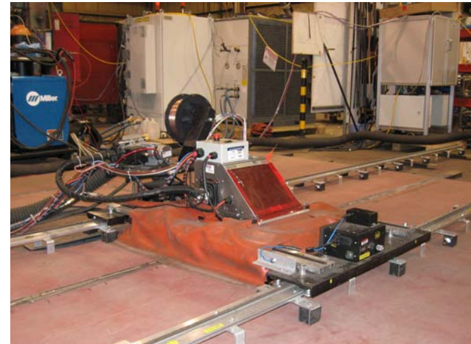
HLAW demonstration system on demonstration panel
