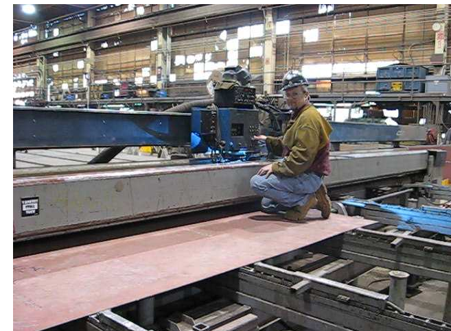
Harding's BIW GMAW Seam Welder, welding TP-3 on 28 January 2008.
