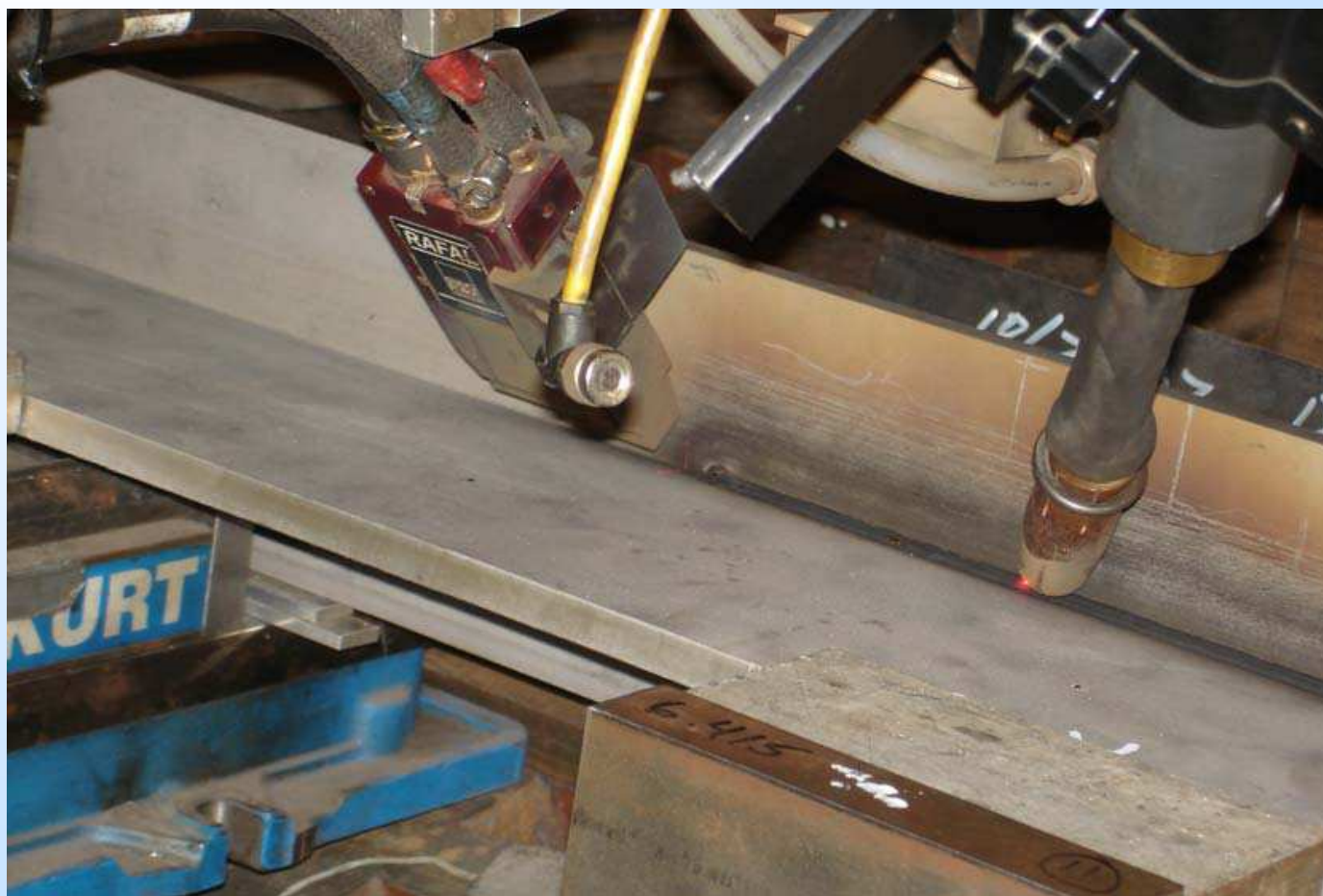
Weld head in position to weld toward left of picture
