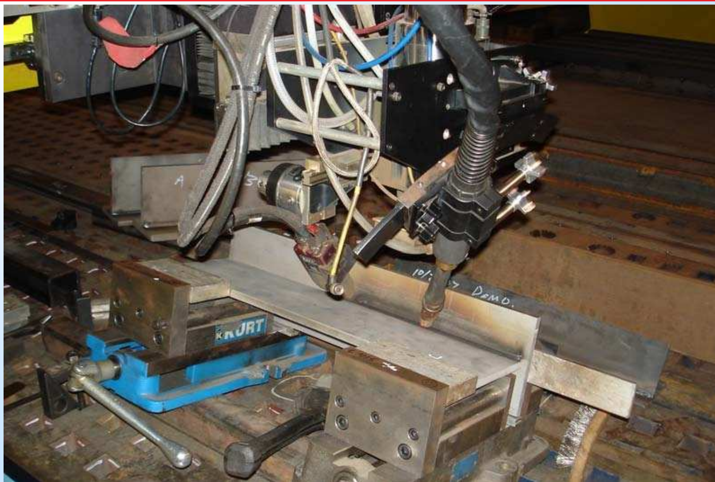
View of Tee in fixture ready for welding
